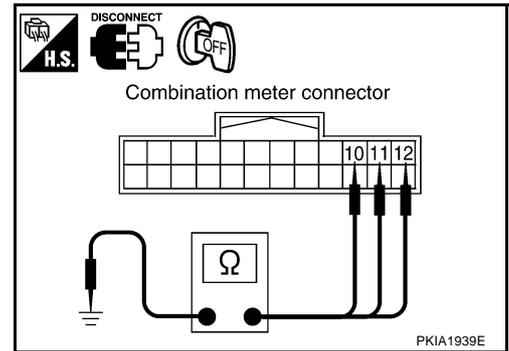
2. Check continuity between unified meter and A/C amp. and ground.
