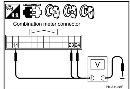
3. Check voltage between unified meter and A/C amp. connector and ground.
