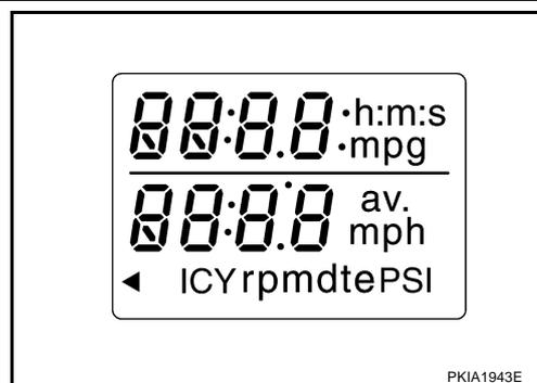
5. Push the odo/trip meter switch. Each meter/gauge should indicate as shown in the figure while pushing odo/trip meter switch.
