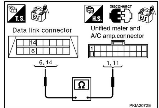
**Circuit Check Between Unified Meter and A/C Amp. and BCM**
