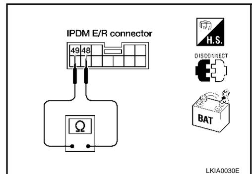
**CAN Communication Circuit Check****1. CHECK CONNECTOR**
