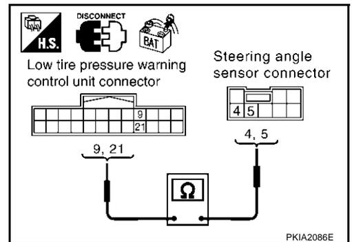
**Circuit Check Between Steering Angle Sensor and VDC/TCS/ABS Control Unit**
