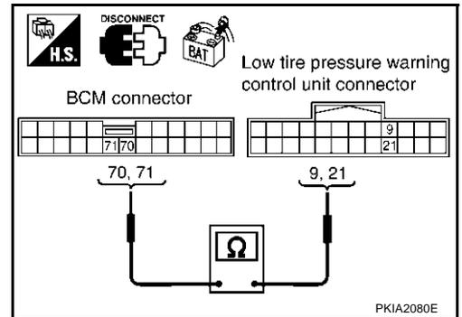
**Circuit Check Between Low Tire Pressure Warning Control Unit and ABS Actuator and Electric Unit (Control Unit)**
