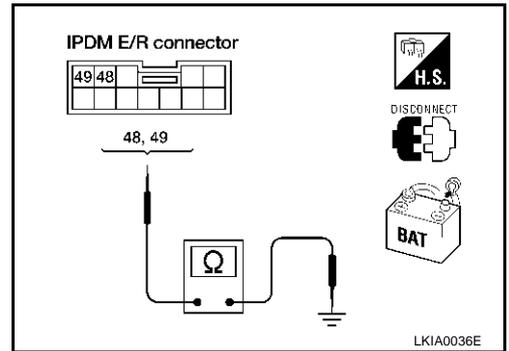
**8. ECM/IPDM E/R INTERNAL CIRCUIT INSPECTION**
