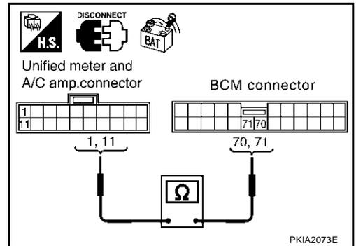
**Circuit Check Between BCM and Low Tire Pressure Warning Control Unit**
