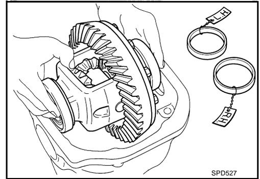
3. Insert left and right side bearing adjusting washer in place between side bearings and carrier.
