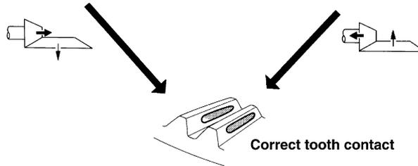
When adjustment is completed, be sure to wipe off completely the ferric oxide and oil or their equivalent.
