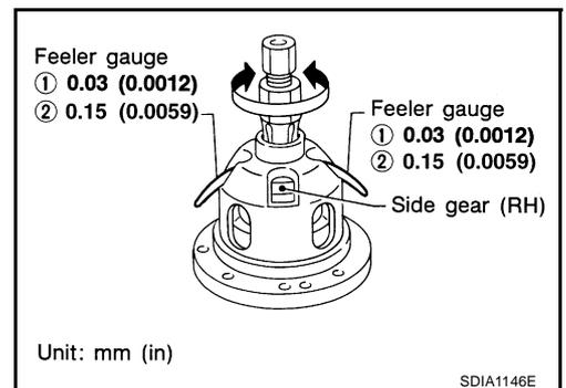
For quiet and reliable final drive operation, the following five adjustments must be made correctly.
