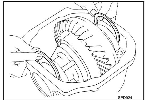
4. Install the side bearing caps in their correct locations and torque the bearing cap retaining bolts.
