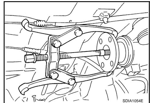
5. Using the side bearing outer race puller, remove oil seal.
