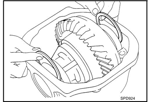
4. Align mark on bearing cap with that on gear carrier and install bearing cap on gear carrier.
