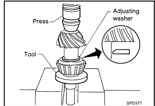
4. Set drive pinion assembly (as shown in figure) in differential carrier and install drive pinion, with press and suitable tool. Stop when drive pinion touches bearing. Apply multi-purpose grease to pinion rear bearing inner race and pinion front bearing inner race.
