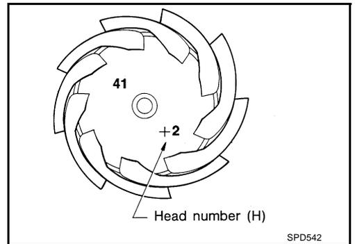
There are two numbers painted on the drive pinion gear. The first one refers to the drive pinion and ring gear as a matched set. This number should be the same as the number on the ring gear. The second number is the "pinion head height number". It refers to the ideal pinion height from standard for quietest operation. Use the following chart to determine the correct pinion height washer.
