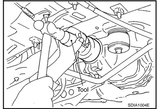
2. Align the matching mark of drive pinion with the matching mark B of companion flange, then install the companion flange.
