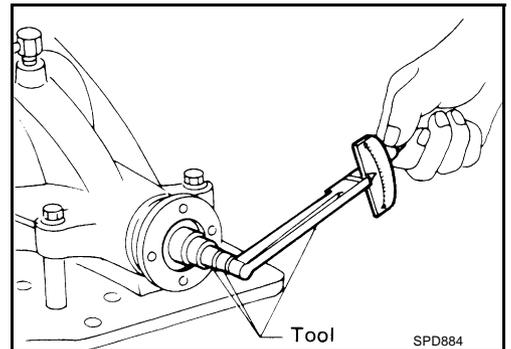
When checking preload, turn drive pinion in both directions several times to seat bearing rollers correctly.
