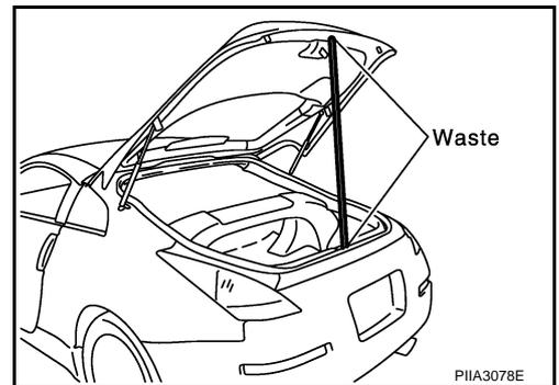
2. Remove stud balls on back door.
