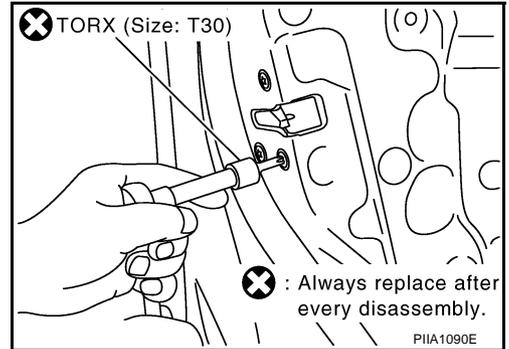
7. Remove the outside handle mounting bolts, remove the outside handle.
