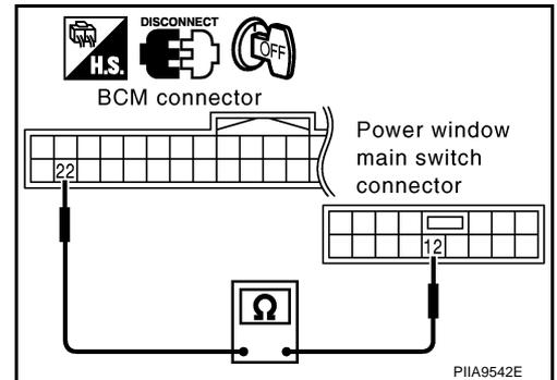
3. Check continuity between BCM harness connector M90 terminal 22 and power window sub-switch (door lock and unlock switch) harness connector D37 terminal 16.
