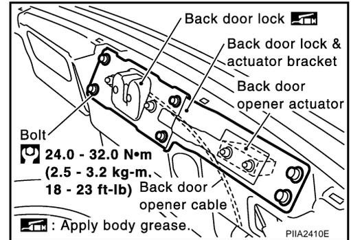
5. Disconnect the connector of the back door opener actuator and back door opener cable, remove the bracket.
