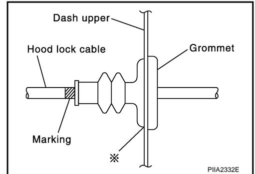
5. Install the hood lock cable securely to the hood lock.
