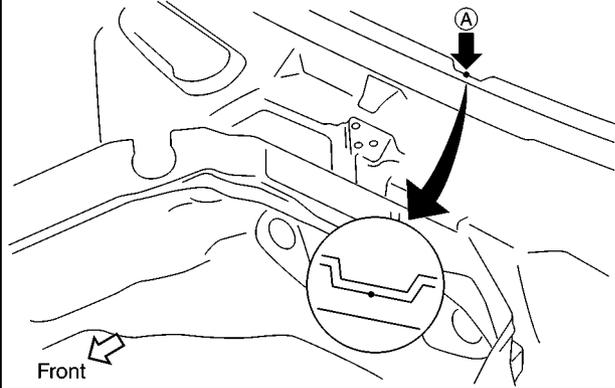
(B) : Front roof flange end of center positioning mark
