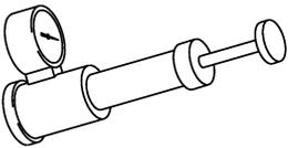
Checking radiator and radiator cap |
