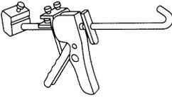
Pressing the tube of liquid gasket                                                                                                                                             |
