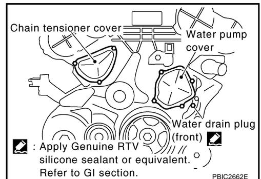
6. Remove chain tensioner cover and water pump cover from front timing chain case.
