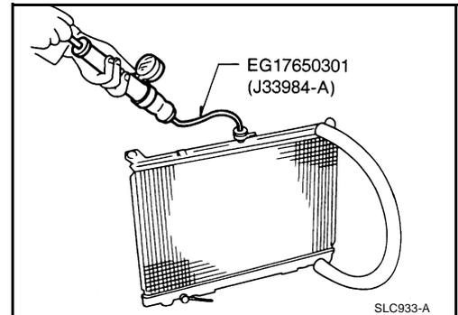
2. Check for leakage by soaking radiator in water container with the testing pressure applied.
