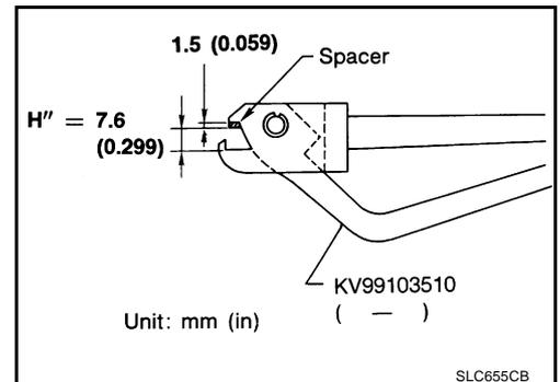
2. Make sure that when radiator plate pliers A [SST: KV99103510 ( — )] are closed dimension H'' is approx. 7.6 mm (0.299 in).
