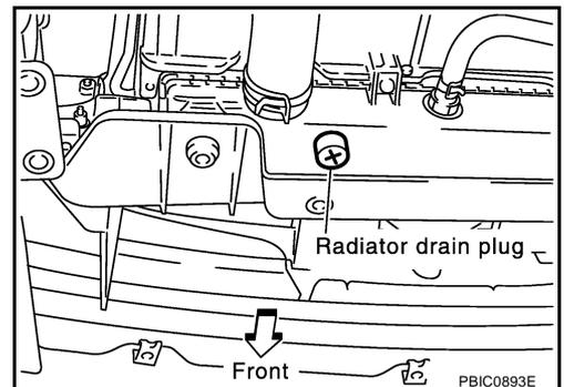
When drain all of engine coolant in the system, open water drain plugs on engine cylinder block. Refer to [EM-112, "DISASSEMBLY"](#) .
