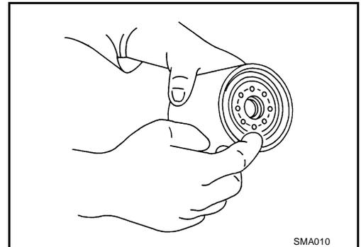
3. Screw oil filter manually until it touches the installation surface, then tighten it by 2/3 turn. Or tighten to specification.
