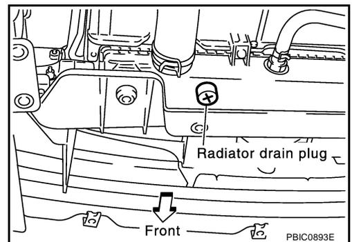
When drain all of engine coolant in the system, open water drain plugs on engine cylinder block. Refer to [EM-112, "DISASSEMBLY"](#).
