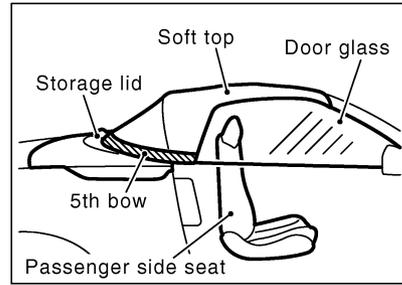
1. Passenger seatback tilts forward by approximately 6° as soon as windows go down, when soft top switch has been pushed on OPEN.
