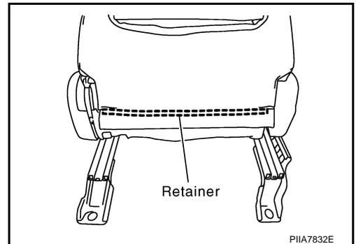
10. After removing the seatback trim and pad, remove the hog rings to separate the trim and pad.
