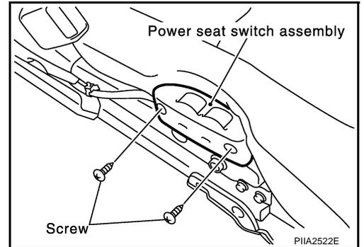
Insert a screwdriver in lower side of power seat switch and remove it (passenger seat for coupe).
