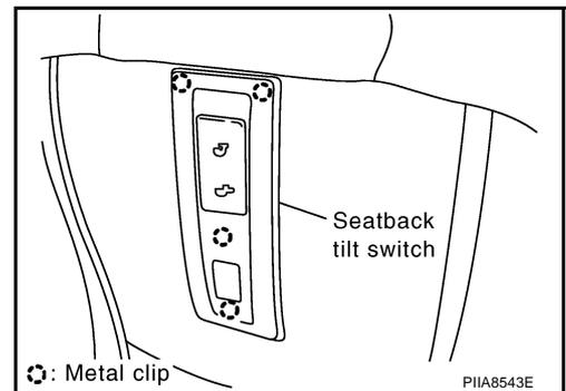
2. Disconnect seatback tilt switch harness connector.
