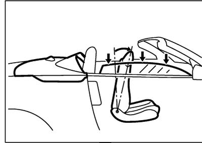
2. Soft top CLOSE operation starts as soon as the passenger seatback tilt forward operation completes.
