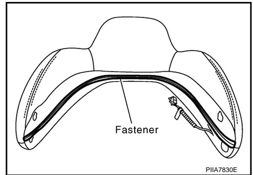
7. Remove the stay securing the inner cloth.
