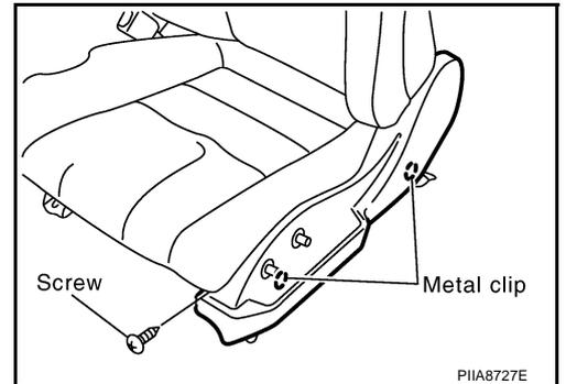
3. Unfasten screws and remove the power seat switch assembly.
