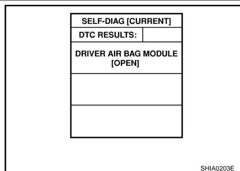
If no malfunction is detected on "SELF-DIAG [CURRENT]" even though malfunction is detected in "SRS Operation Check", check the battery voltage. If the battery voltage is less than 9 V, charge or replace the battery. [SRS-28, "DIAGNOSTIC PROCEDURE 3"](#). If the battery voltage is OK, go to [SRS-30, "DIAGNOSTIC PROCEDURE 4 \(CONTINUED FROM DIAGNOSTIC PROCEDURE 2\)"](#) diagnose the following cases:
