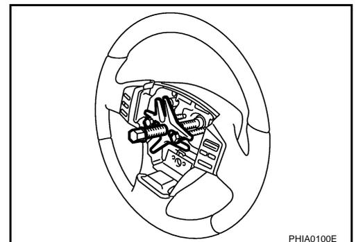
7. Loosen the spiral cable fixing screws, remove the spiral cable.
