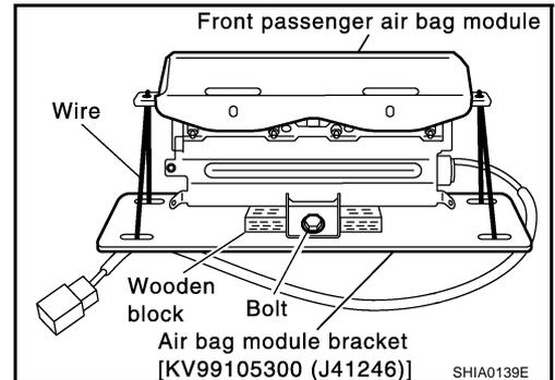
3. Connect deployment tool [SST: KV99106400 (J38381)] and deployment tool adapter (SST: J38381-65) to front passenger air bag module connector.
