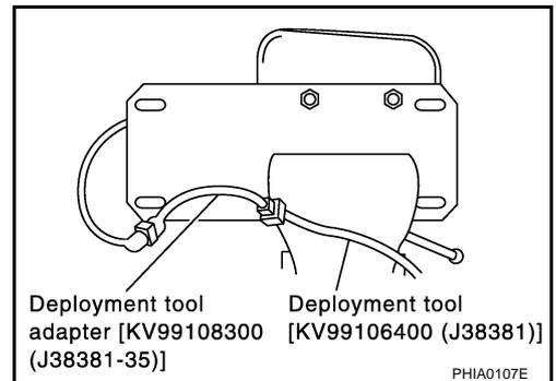
5. Connect red clip of deployment tool to battery positive terminal and black clip to negative terminal.
