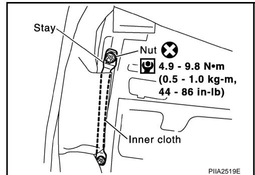
5. Remove the front side air bag module.
