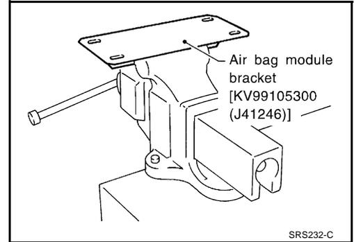
2. Match the hole in air bag module bracket (held in vise) and front passenger air bag module and fix them with one bolt [M8 × 25 - 30 mm (0.98 - 1.18 in)].
