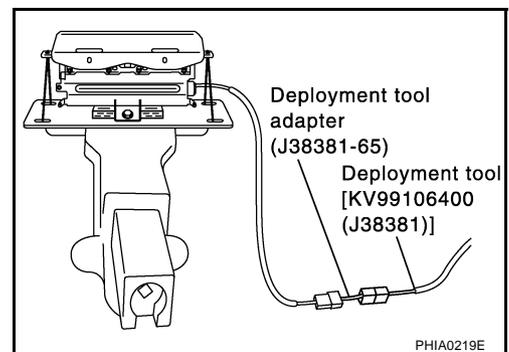
6. Press the button on the deployment tool. The left side lamp on the tool, marked "air bag connector voltage", will illuminate and the air bag module will deploy.
