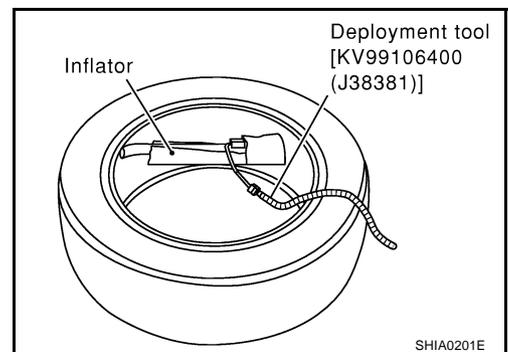
4. Put the tire with the inflator onto another tire without wheel. Add an additional tire without a wheel and then a tire mounted on a wheel on top.
