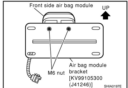
4. Connect deployment tool adapter [SST: KV99108300 (J38381-35)] and deployment tool [SST: KV99106400 (J38381)] on side air bag module.
