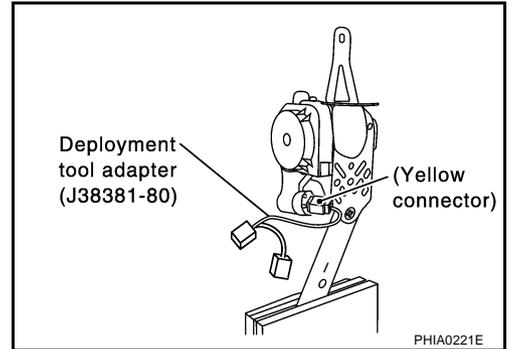
3. Connect red clip of deployment tool to battery positive terminal and black clip to negative terminal.
