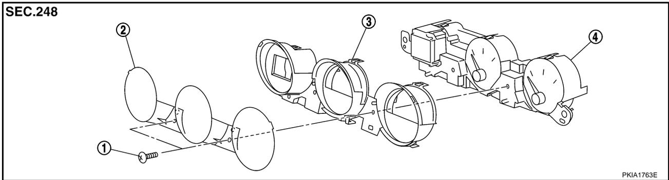
1. Remove screws (2), and remove front cover.
