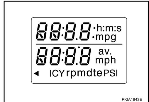
5. Push the odo/trip meter switch. Each meter/gauge should indicate as shown in the figure while pushing odo/trip meter switch.
