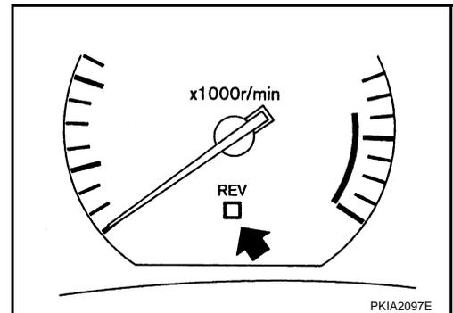
between 2,000 and 8,000 rpm by pressing trip computer setting switch for less than approximately 1 second will add the figure by 100 rpm. If pressing for more than approximately 1 second, the figure will increase by 500 rpm.
