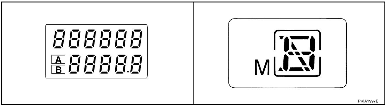
7. Push the odo/trip meter switch. Each meter/gauge should indicate as shown in the figure while pushing odo/trip meter switch. (at this time, the low-fuel warning lamp goes off).
