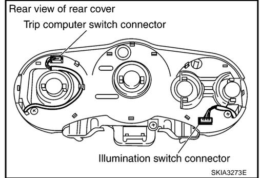
5. Remove screws (2) and remove rear cover.
