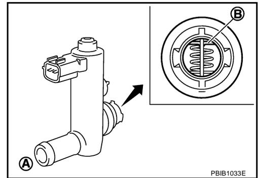
3. Check air passage continuity and operation delay time under the following conditions.
