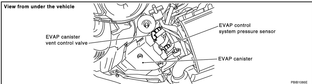
2. Check sensor harness connector for water.
