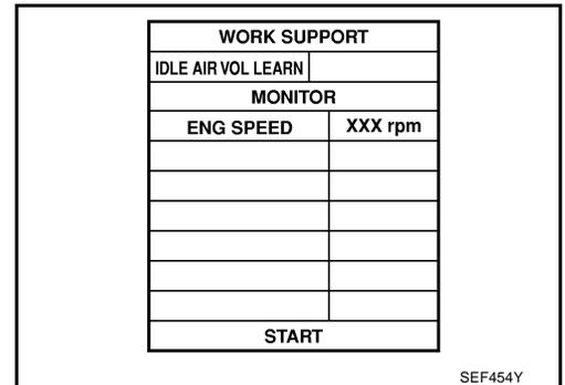
7. Make sure that "CMPLT" is displayed on CONSULT-II screen. If "CMPLT" is not displayed, Idle Air Volume Learning will not be carried out successfully. In this case, find the cause of the incident by referring to the Diagnostic Procedure below.
