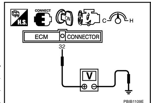
8. Verify that EVAP control system pressure sensor value stays 0.1V less than the value at idle speed (measured at step 6) for at least 1 second.
