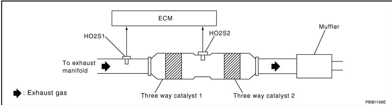
A three way catalyst 1 with high oxygen storage capacity will indicate a low switching frequency of heated oxygen sensor 2. As oxygen storage capacity decreases, the heated oxygen sensor 2 switching frequency will increase.
