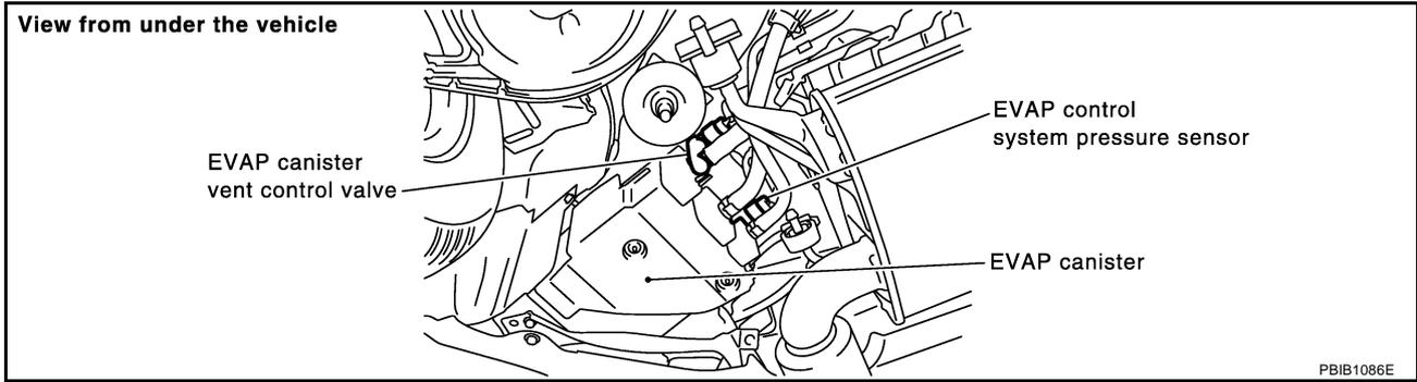
4. To locate the leak, deliver positive pressure to the EVAP system until pressure gauge points reach 1.38 to 2.76 kPa (0.014 to 0.028 kg/cm<sup>2</sup> , 0.2 to 0.4 psi).
