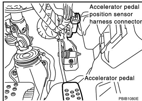
3. Check voltage between APP sensor terminal 6 and ground with CONSULT-II or tester.
