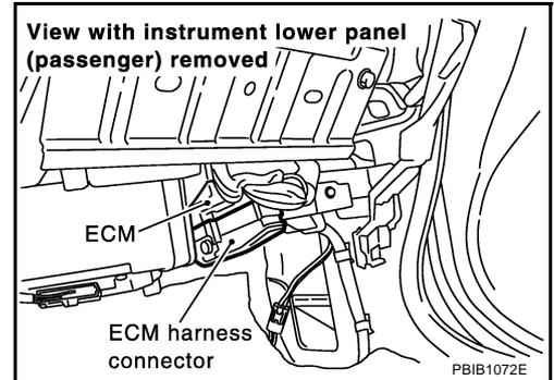
3. When disconnecting ECM harness connector, loosen it with levers as far as they will go as shown in the figure.
