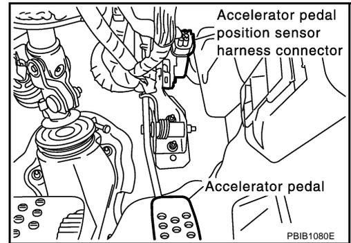
3. Check voltage between APP sensor terminal 4 and ground with CONSULT-II or tester.
