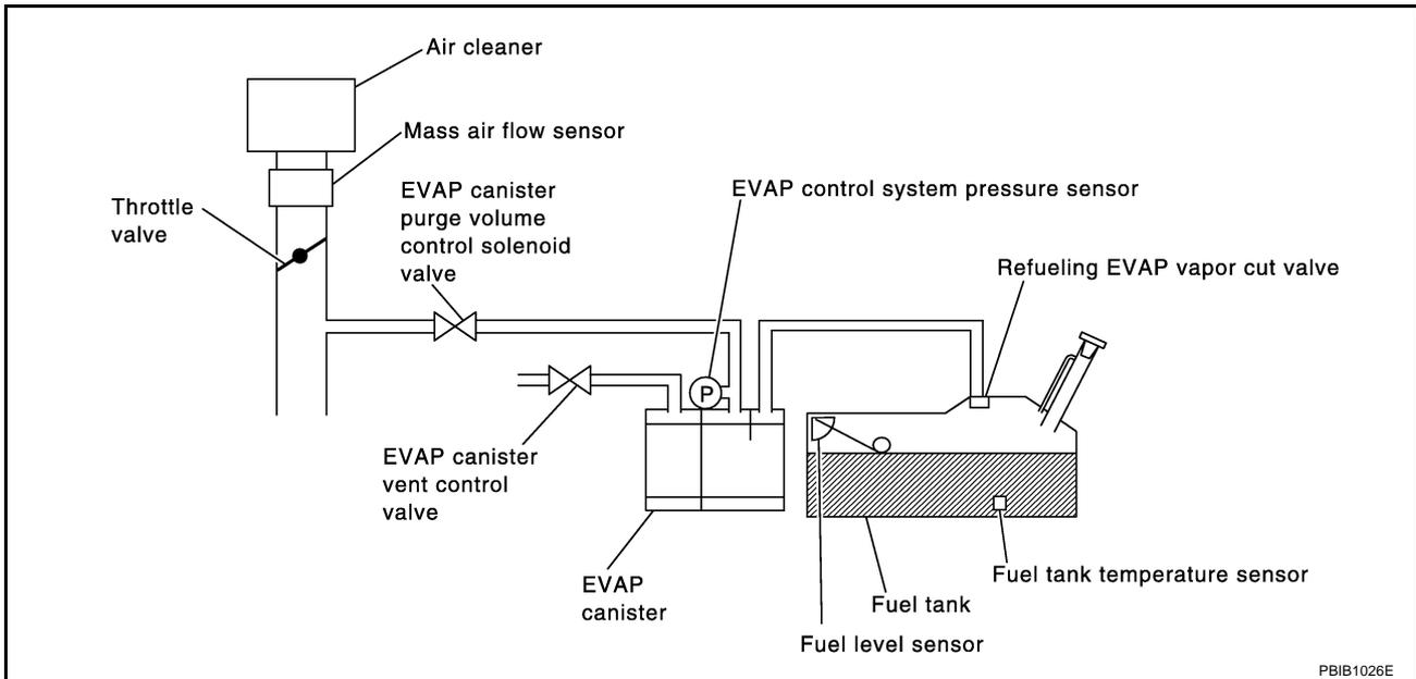
In this evaporative emission (EVAP) control system, purge flow occurs during non-closed throttle conditions. Purge volume is related to air intake volume. Under normal purge conditions (non-closed throttle), the EVAP canister purge volume control solenoid valve is open to admit purge flow. Purge flow exposes the EVAP control system pressure sensor to intake manifold vacuum.
