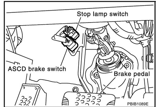
2. Check voltage between stop lamp switch terminal 1 and ground with CONSULT-II or tester.
