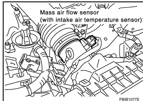
4. Check voltage between mass air flow sensor terminal 5 and ground.
