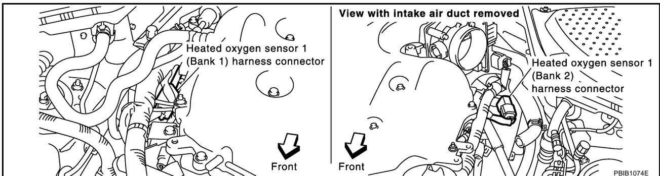
3. Check harness continuity between HO2S1 terminal 4 and ECM terminal 78. Refer to Wiring Diagram.
