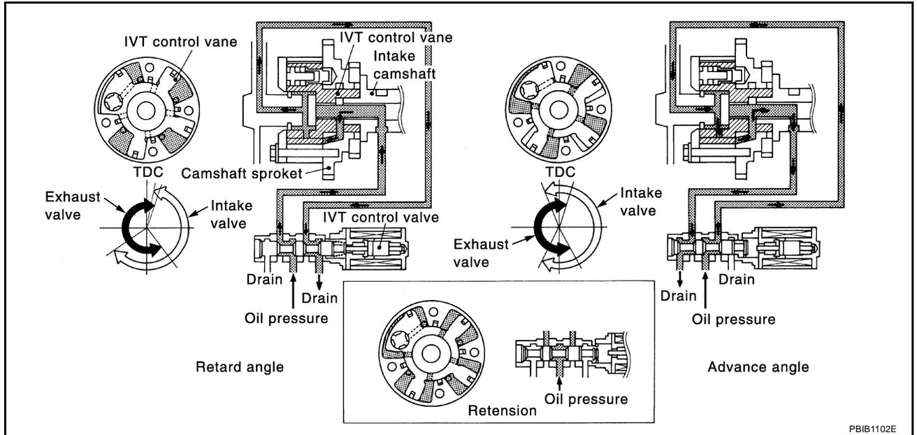
This mechanism hydraulically controls cam phases continuously with the fixed operating angle of the intake valve.
