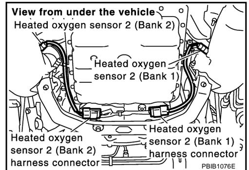
4. Check voltage between HO2S2 terminal 2 and ground with CONSULT-II or tester.
