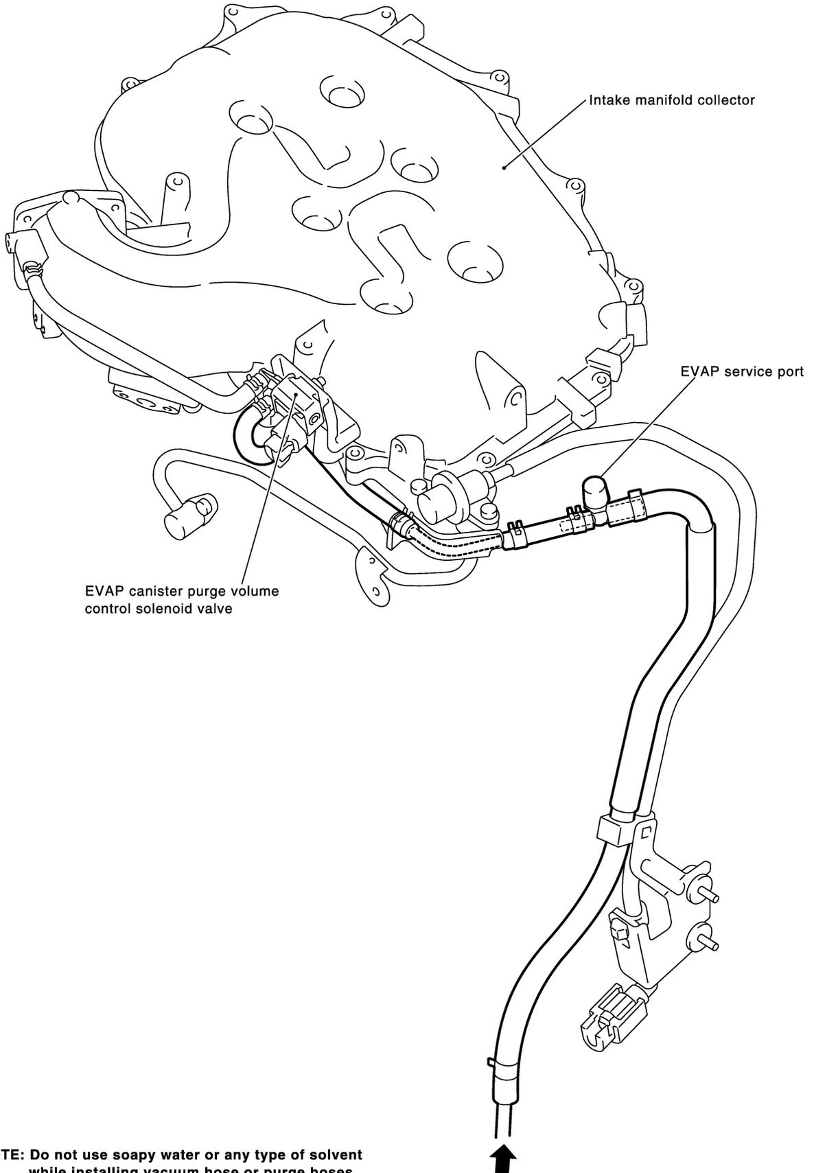
**NOTE: Do not use soapy water or any type of solvent while installing vacuum hose or purge hoses.**
