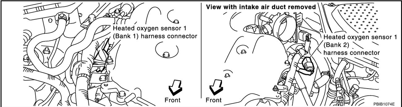
4. Check harness continuity between HO2S1 terminal 4 and ECM terminal 78. Refer to Wiring Diagram.
