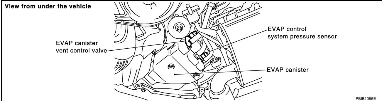
3. Pressurize the EVAP line using pressure pump with 1.3 to 2.7 kPa (10 to 20 mmHg, 0.39 to 0.79 inHg), then remove pump and EVAP service port adapter.
