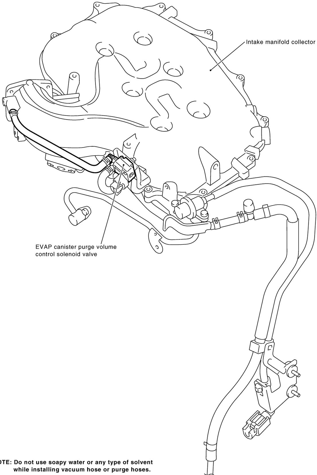
EVAP canister purge volume control solenoid valve
