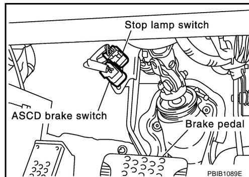
3. Check voltage between stop lamp switch terminal 1 and ground with CONSULT -II or tester.
