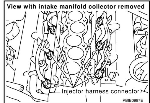
4. Check voltage between injector terminal 1 and ground with CONSULT-II or tester.
