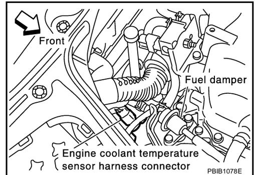
4. Check voltage between ECT sensor terminal 1 and ground with CONSULT-II or tester.
