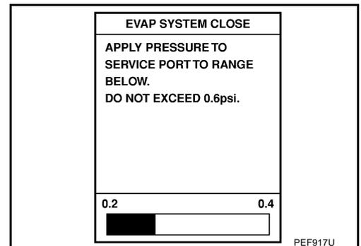
4. Using EVAP leak detector, locate the EVAP leak. For the leak detector, refer to the instruction manual for more details.
