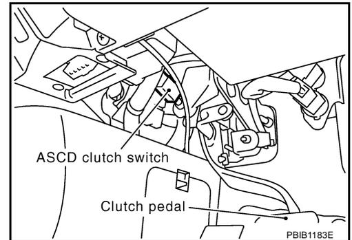
4. Check voltage between ASCD clutch switch terminal 1 and ground with CONSULT-II or tester.
