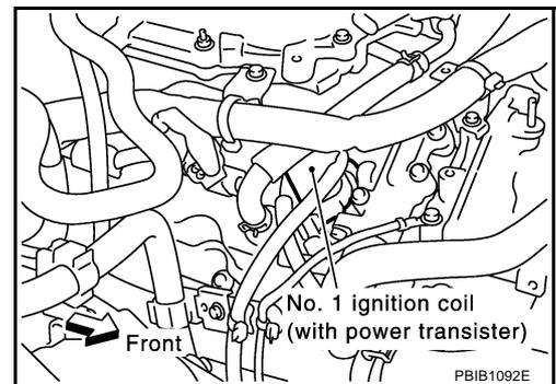
2. Connect No. 1 ignition coil and No. 1 spark plug with suitable high-tension wire as shown, and attach timing light clamp to this wire.
