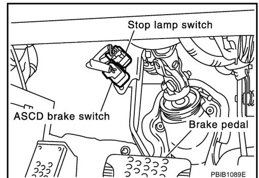
3. Check voltage between stop lamp switch terminal 1 and ground with CONSULT -II or tester.
