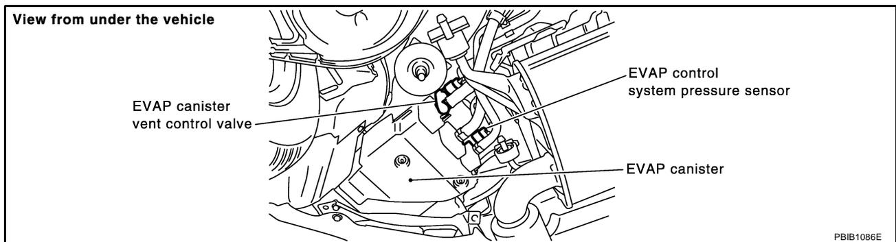
2. Check sensor harness connector for water.
