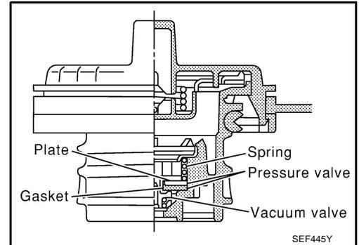
2. Check valve opening pressure and vacuum.
