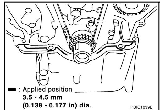
c. Assemble front timing chain case.
