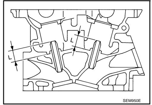
6. Using valve guide reamer, apply reamer finish to valve guide.
