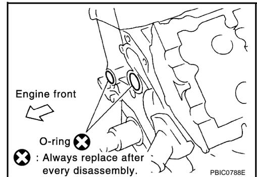
3. Install O-rings to cylinder head.
