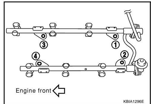
8. Remove fuel injector from fuel tube with following procedure.
