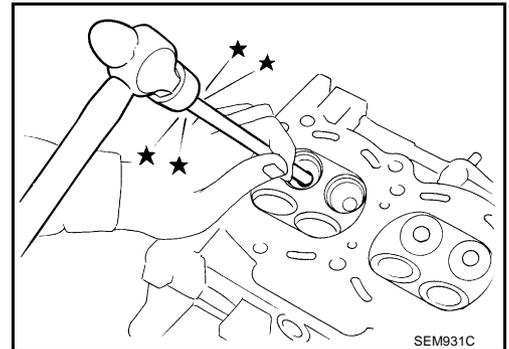
3. Using valve guide reamer, ream cylinder head valve guide hole.
