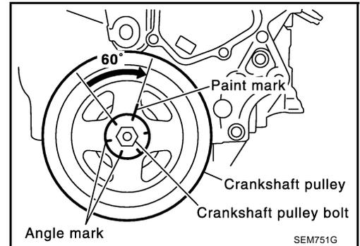
10. Rotate crankshaft pulley in normal direction (clockwise when viewed from front) to confirm it turns smoothly.
