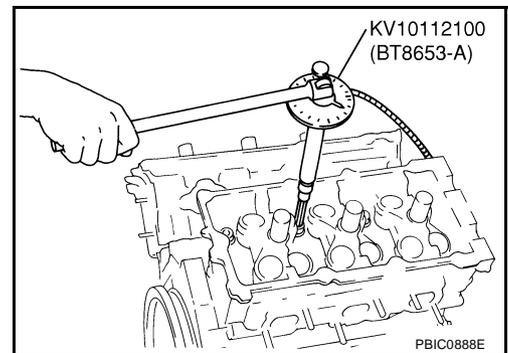
4. After installing cylinder head, measure distance between front end faces of cylinder block and cylinder head (left and right banks).
