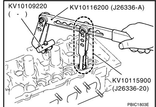
5. Remove valve oil seal using valve oil seal puller (special service tool).
