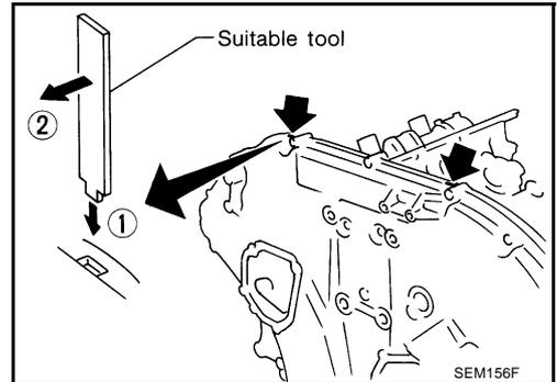
18. Remove water pump cover and chain tensioner cover from front timing chain case.
