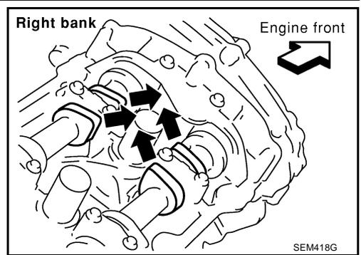
13. Remove starter motor and set ring gear stopper (special service tool) as shown. Refer to [SC-19, "Removal and Installation"](#).
