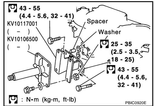
5. Lift engine, and mount it onto the engine stand.
