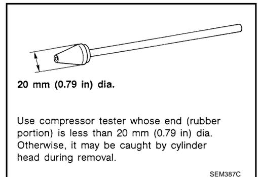
8. With accelerator pedal fully depressed, turn ignition switch to "START" for cranking. When the gauge pointer stabilizes, read the compression pressure and engine rpm. Perform these steps to check each cylinder.
