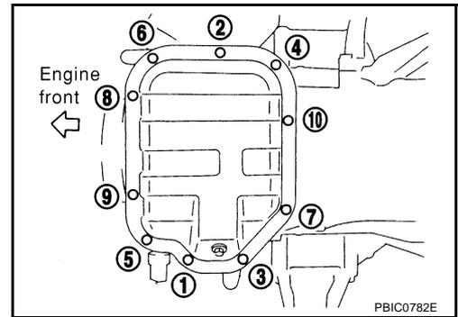
4. Install oil pan drain plug.
