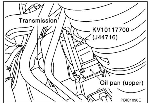
19. Remove crankshaft pulley.
