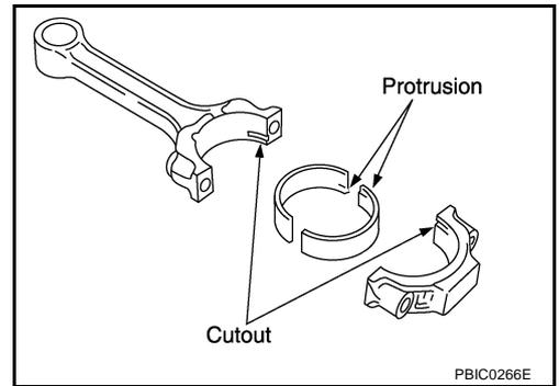
14. Install piston and connecting rod assembly to crankshaft.
