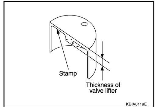
Available thickness of valve lifter: 27 sizes with range 7.88 to 8.40 mm (0.3102 to 0.3307 in) in steps of 0.02 mm (0.0008 in) (when manufactured at factory).
