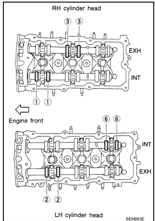
c. Rotate crankshaft by 240° clockwise (when viewed from front) to align No. 3 cylinder at TDC of its compression stroke.
