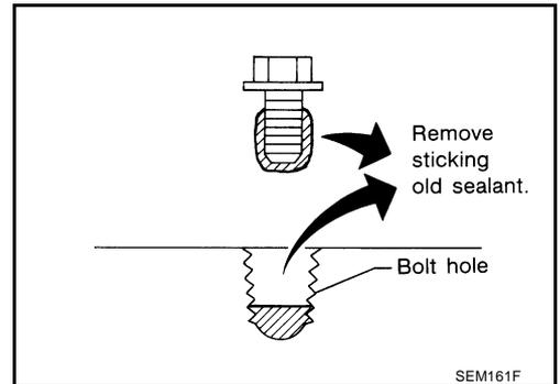
32. Use a scraper to remove all traces of liquid gasket from water pump cover, chain tensioner cover and intake valve timing control covers.
