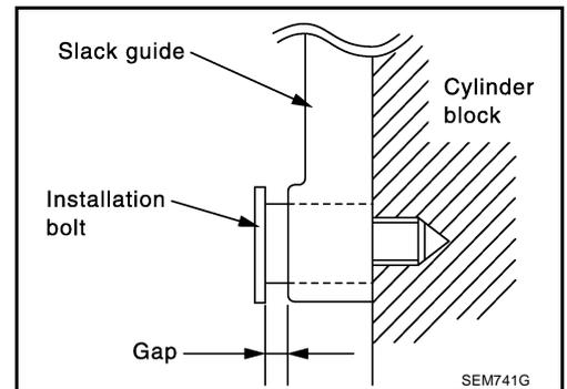
15. Install chain tensioner for slack guide.
