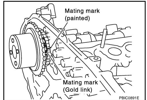
10. After confirming the mating marks are aligned, tighten camshaft sprocket mounting bolts.
