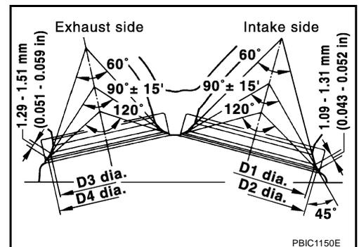
6. Using compound, grind to adjust valve fitting.
