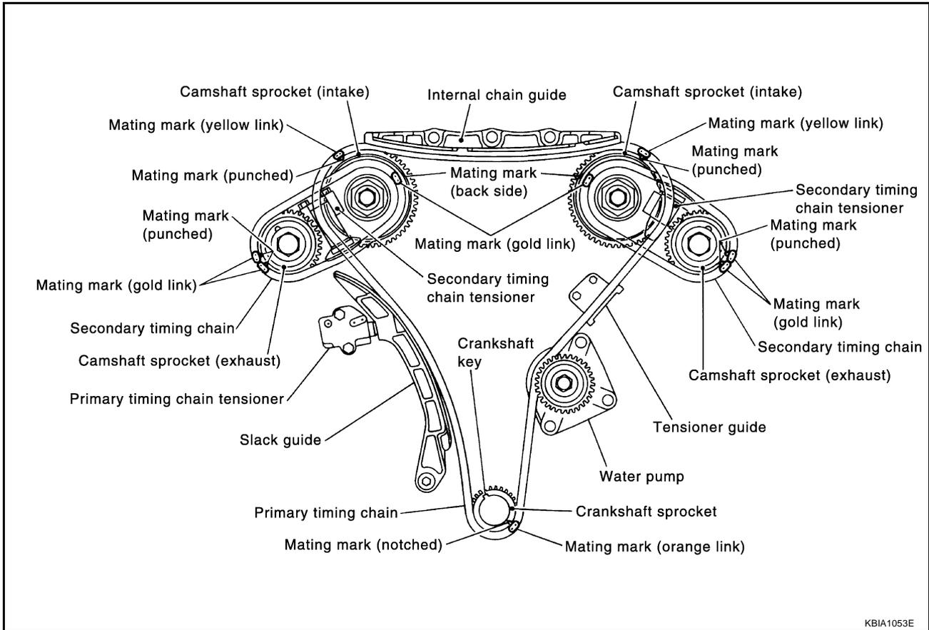
1. Install RH and LH secondary timing chain tensioners to cylinder head as follows if removed. Refer to [EM-69, "INSTALLATION"](#).
