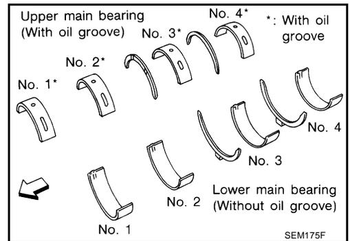
5. Install crankshaft to cylinder block.
