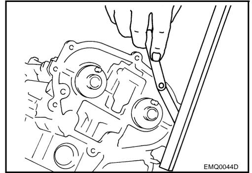
7. Inspect and adjust valve clearance. Refer to [EM-72, "Valve Clearance"](#).
