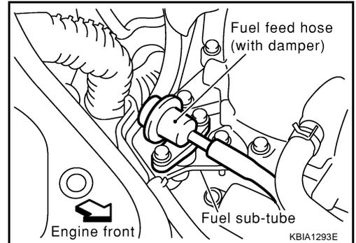
4. When separating fuel feed hose (with damper) and centralized under-floor piping connection, disconnect quick connector with the following procedure.
