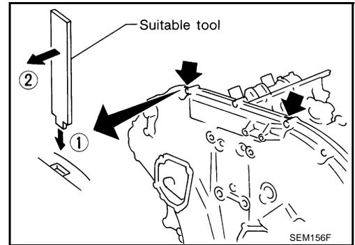
21. Remove water pump cover and chain tensioner cover from front timing chain case.
