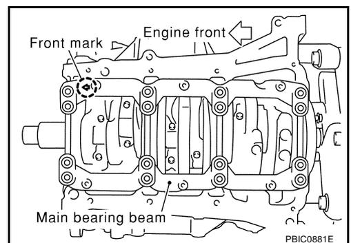
9. Install main bearing cap bolt.
