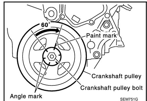
24. Rotate crankshaft pulley in normal direction (clockwise when viewed from front) to confirm it turns smoothly.
