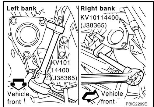
10. Remove exhaust manifold cover.
