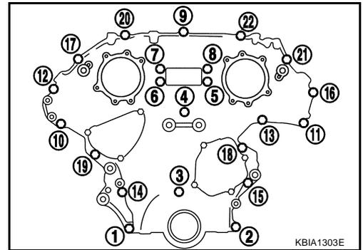
7. Install two mounting bolts in front of oil pan (upper) in numerical order shown in the figure.
