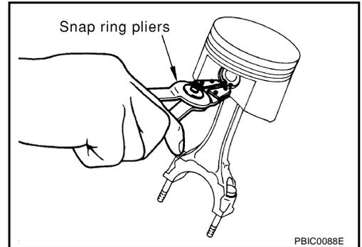
b. Heat piston to 60 to 70°C (140 to 158°F) with drier or equivalent.
