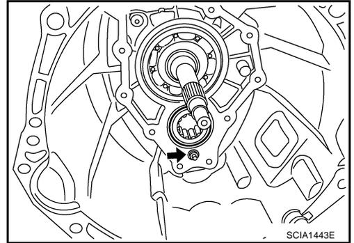
19. Remove snap ring from the main drive gear bearing, using snap ring pliers.
