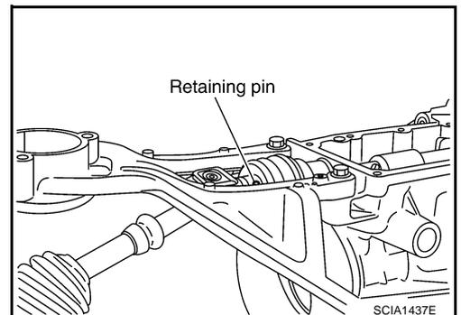
6. Remove control bracket mounting bolts. Then remove check shift pin and control bracket as one unit from the rear extension.
