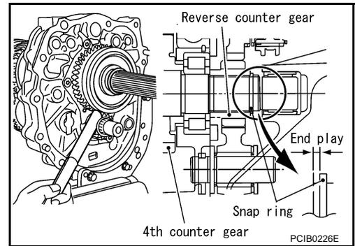
1. After removing snap ring and reverse coupling snap ring, using puller to remove reverse main gear and reverse synchronizer assembly.
