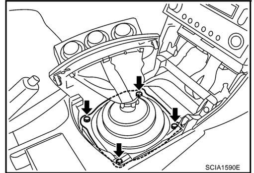
11. Remove guide plate mounting bolts and then separate shift lever assembly from the shift lever housing assembly.
