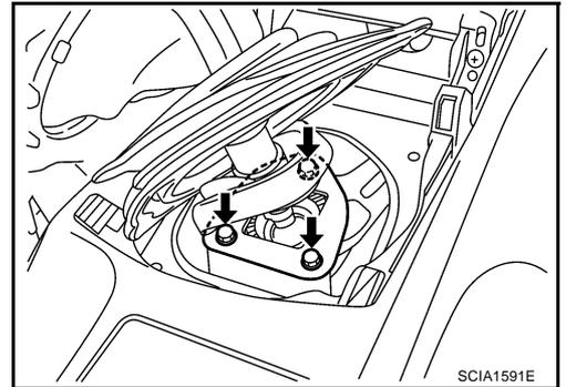
12. Remove clutch operating cylinder mounting bolts and then separate clutch operating cylinder from the transmission case.
