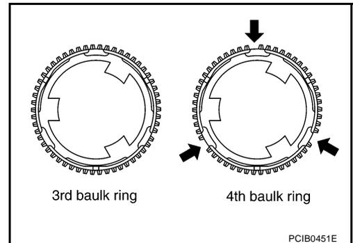
17. Install 4th outer baulk ring, 4th synchronizer cone, 4th inner baulk ring, 4th needle bearing, and 4th counter gear onto the counter shaft and then using the inserter and a press to press fit the 4th gear bushing and 4th counter gear thrust washer.
