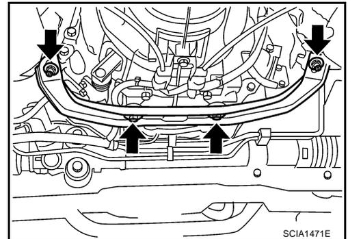
5. Remove nut connecting catalytic converter to exhaust manifold, and then remove catalytic converter and exhaust front tube as one unit.
