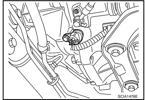
16. Remove starter motor. Refer to [SC-19, "Removal and Installation"](#).
