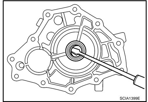
18. Remove baffle plate mounting nut from the transmission case.
