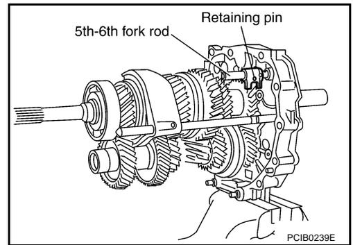
17. Using a pin punch [6 mm (0.24 in) dia.] to knock out retaining pin, and then remove 5th - 6th fork rod (reversal side) and 5th - 6th shift fork.
