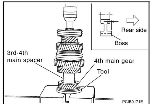
10. Install 3rd - 4th main spacer on the main shaft and then using the inserter and a press to press fit the 4th main gear.
