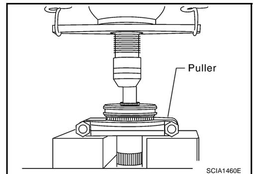
19. Using a press to remove the 3rd counter gear, 3rd - 4th synchronizer assembly, 4th counter gear, 4th needle bearing, 4th gear bushing, 4th counter gear thrust washer, and counter rear bearing inner race.
