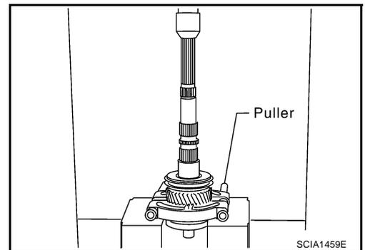
17. After removing snap ring, using a press to remove 6th main gear and 5th - 6th synchronizer assembly.
