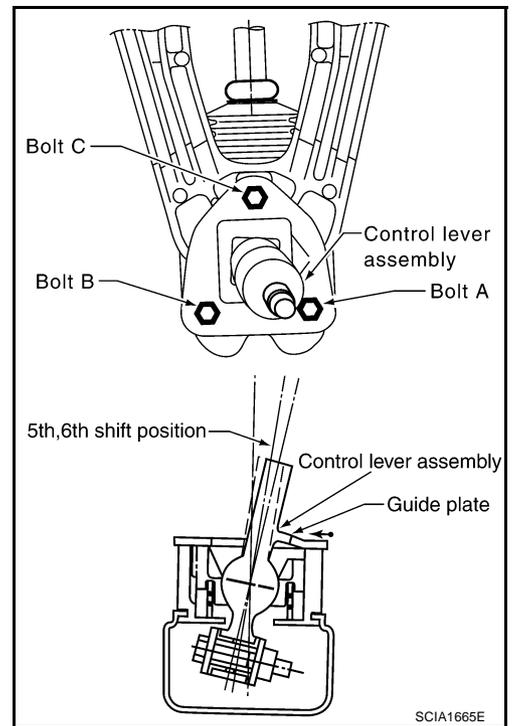
5. Shifting control lever assembly to 5th gear, the control lever assembly light pressed to the reverse side.
