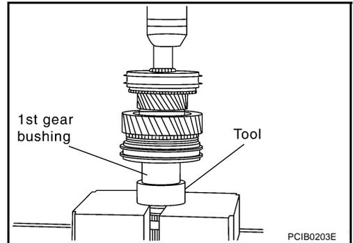
9. Install 1st outer baulk ring, 1st synchronizer cone, 1st inner baulk ring, 1st needle bearing, and 1st main gear on the main shaft and then using the inserter and a press to press fit the 3rd main gear.
