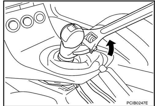
2. Loosen the shift knob to remove the control lever.
