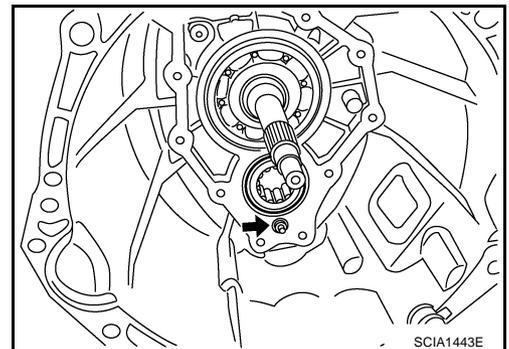
7. Apply multi-purpose grease to the lip of the front cover oil seal. Using a drift, to install oil seal approx. 8.55-9.55 mm (0.336-0.376 in) above from the front cover edge surface.
