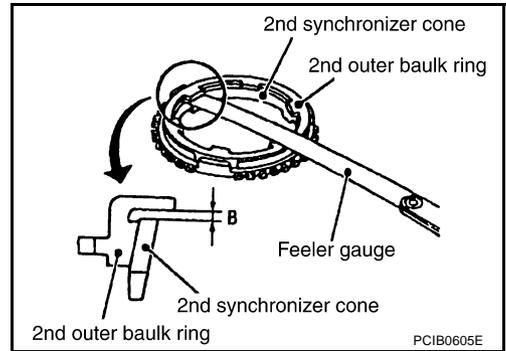
3. Using filler gauge put and press baulk ring on 2nd main gear taper cone, and then measure "clearance C" at more than 2 diagonal points, and calculate the average.
