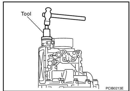
16. Apply multi - purpose grease to the lip of the rear oil seal. Using a drift to install rear oil seal. 1.2-2.2 mm (0.047-0.87 in) above from the rear extension edge surface.
