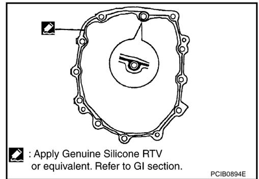
18. Install rear extension to the adapter plate and then tighten mounting bolts to the specified torque in order as shown on the figure.
