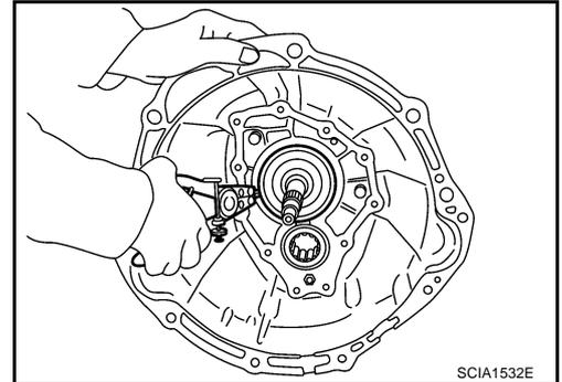
6. Tighten baffle plate mounting nut to the specified torque.
