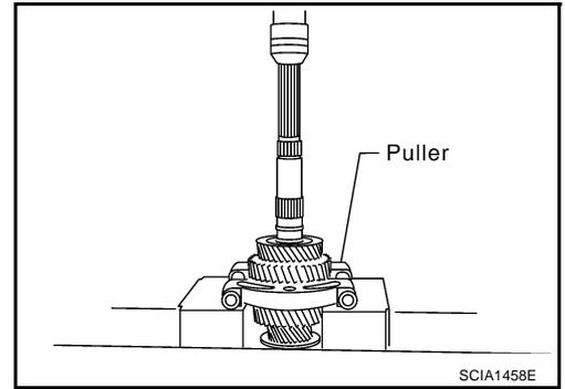
15. Using a press to remove 1st gear bushing, 1st - 2nd synchronizer assembly, and 2nd main gear.
