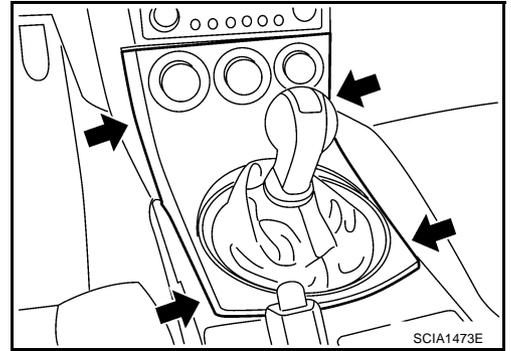
9. Remove hole cover mounting bolts and then separate hole cover from the floor panel.
