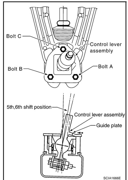
11. As shown in the figure, assemble seat and insulator to control lever assembly.
