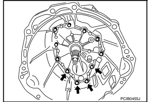
11. Tighten bolts to the specified torque in order as shown on the figure.
