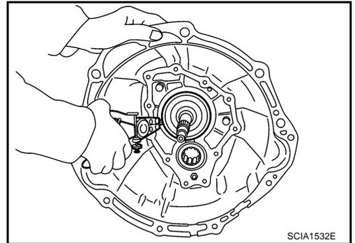
20. Using a soft hammer to carefully tap main shaft and counter shaft from the transmission case side, and then separate adapter plate and transmission case.
