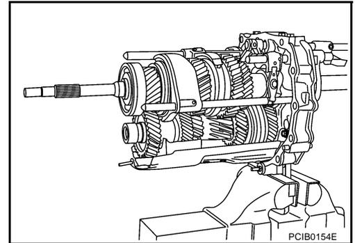
3. Remove magnet from the adapter plate.
