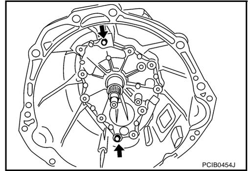
10. Temporary tightening remaining 9 bolts, tighten bolts to the specified torque.
