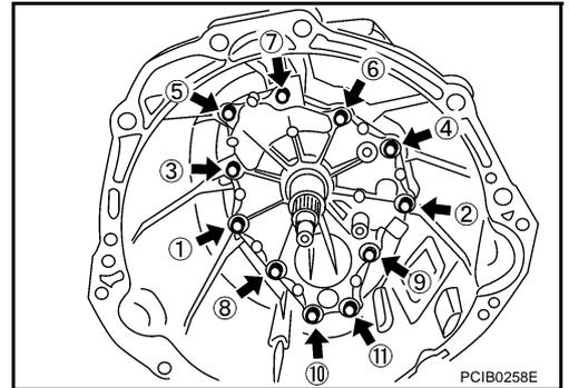
12. Install washer to the withdrawal lever ball pin and then install it to front cover. Tighten withdrawal lever ball pin to the specified torque.
