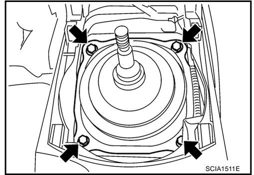
7. Remove guide plate mounting bolts, and then remove control lever assembly and control lever spring.
