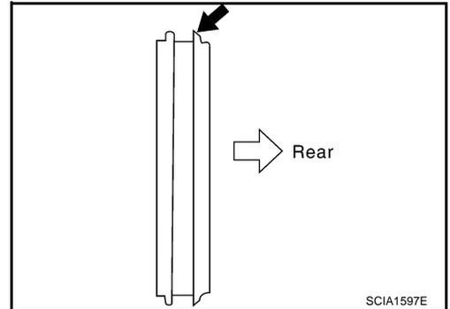
2. Install 5th - 6th spread spring in the 5th - 6th shifting insert.
