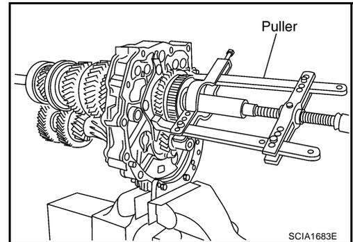
3. Remove main shaft bearing retainer mounting bolts and then remove main shaft bearing retainer.
