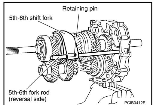
4. Install 5th - 6th fork rod to the adapter plate.
