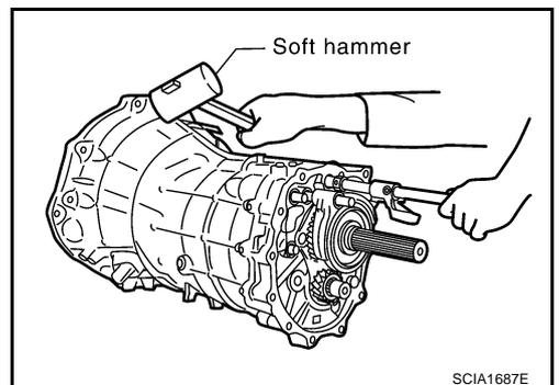
21. Remove counter front bearing from the transmission case.
