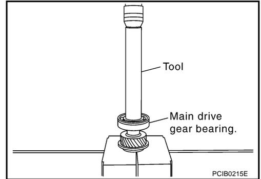
20. Select and install a snap ring to the main drive gear bearing so that the end play comes within the standard value.
