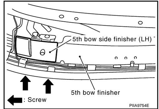
15. Remove 5th bow finisher by pulling the finisher up.
