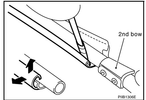
36. Pull up 3rd bow retainer by using a screwdriver, and then remove soft top cover from 3rd bow.
