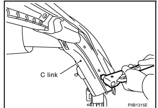
19. Align screw hole on soft top cover and the bottom of C link, and then tighten with screw.
