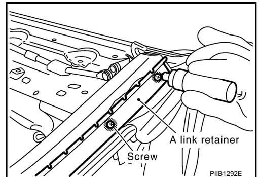
14. Remove screws, and then remove A link retainer.
