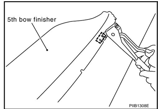
6. Remove remains of soft top cover mounting rivet from 5th bow and C link.
