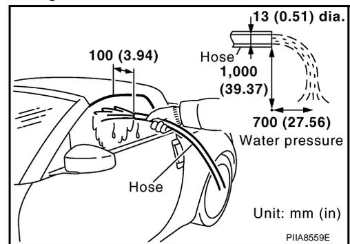
4. Visually check for water leakage.
