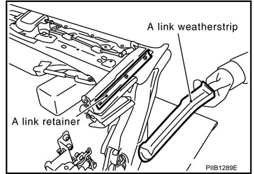
11. Peel a link sealing out.
