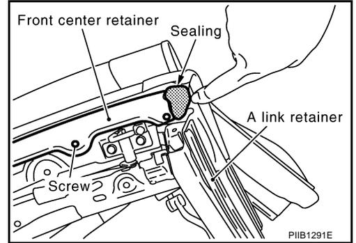
12. Remove screws, and then remove front center retainer.
