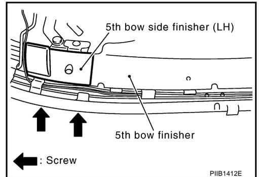
3. Remove clips, and then remove 5th bow finisher.
