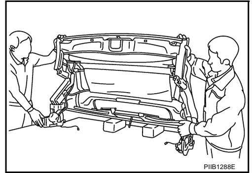
16. Remove clips on the top of C link and 5th bow weatherstrip.
