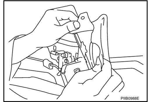
11. Align soft top cover hole and grommet hole at the 1st bow.
