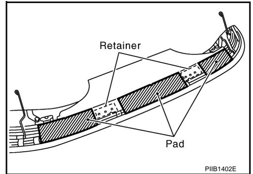
2. Remove screws, and then remove 5th bow side finisher (RH/LH).
