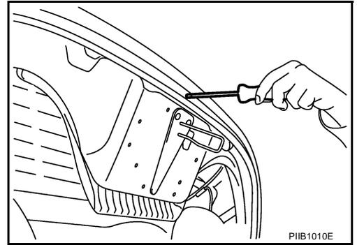
8. Drilling rivets attaching the soft top cover to 5th bow, then pull up the soft top cover bottom edge.
