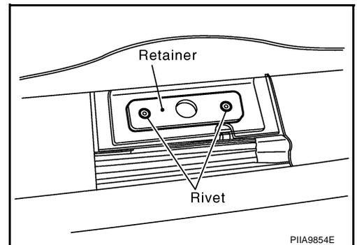
10. Drilling rivets under retainers by using 4 mm (0.16 in) diameter drill bit.
