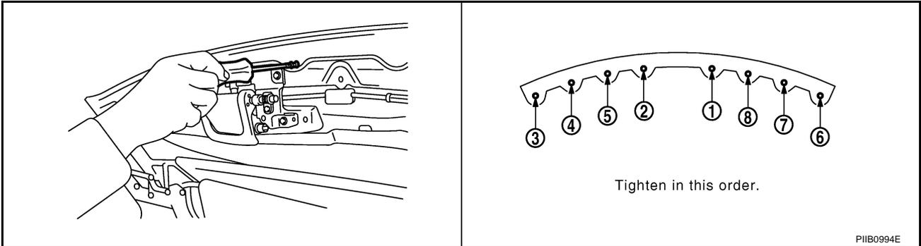
13. Apply EPT seal to A link installation position.
