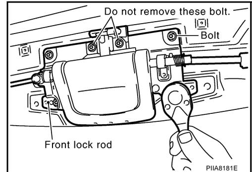
3. Remove bolts, and then remove front lock striker, LH, center, and RH.
