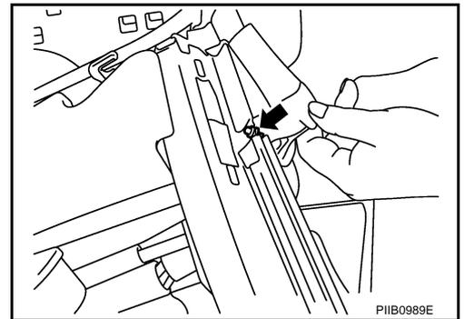
32. Remove soft top cover wire rear bracket from C link.
