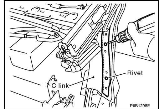
25. Cut EPT seal and remove screws on the bottom of C link.
