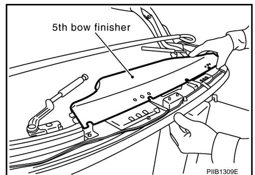
4. Remove rivets head of 5th bow finisher retainer.
