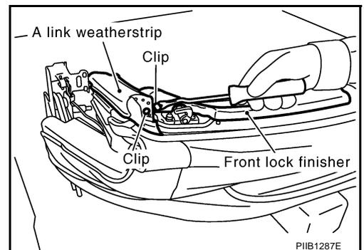
9. Pull up front lock lever, and then disengage clips to remove front lock finisher.
