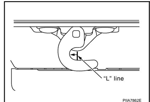
3. Adjust hook contact length by adjusting front lock rod length using front lock rod adjust bolt if "L" line is not exceeded in front lock hook, RH and LH.
