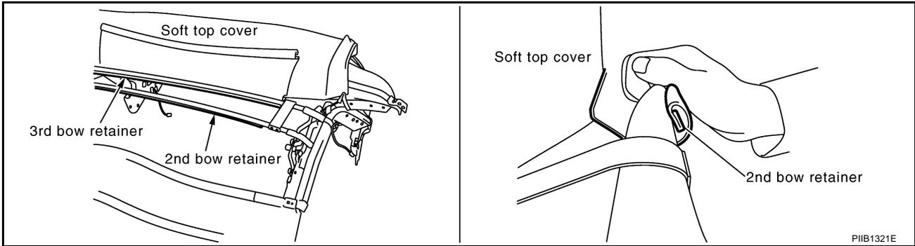
5. Hook soft top cover inner fabric edge to 2nd bow retainer and press retainer to hold securely.
