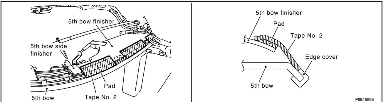
10. Secure 5th bow finisher harness with new nonwoven fabric if necessary.
