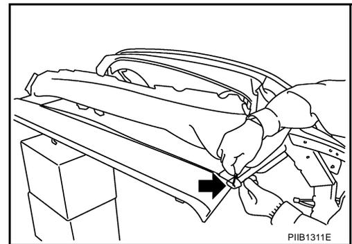
8. Tighten soft top cover wire rear bracket to C link with screw.
