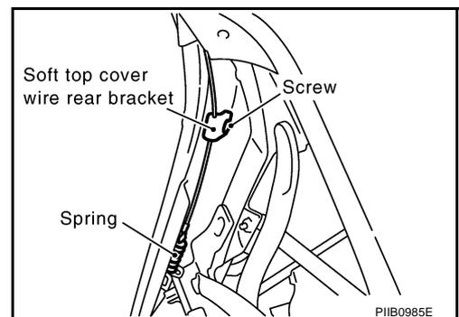
9. Hook soft top cover wire spring on C link and bend the hook of wire spring to prevent unhooking the hook.
