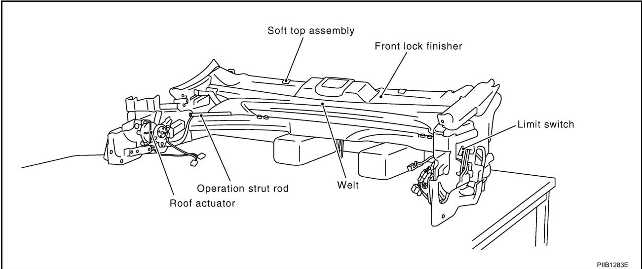
3. Remove roof actuator (RH/LH). Refer to [RF-107, "Removal and Installation of Roof Actuator"](#).
