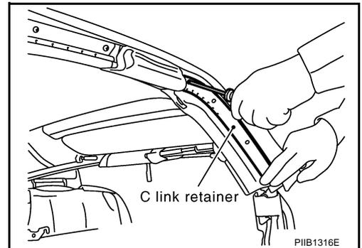
22. Apply seal to C link lower installation position.
