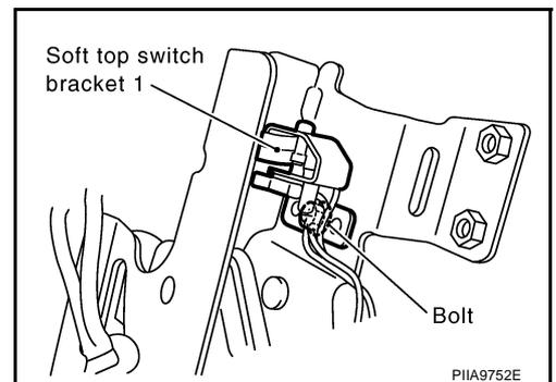
5. Remove limit switches with soft top switch bracket 2 by removing bolt.
