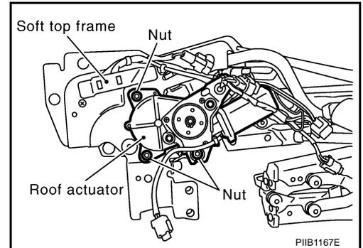
3. Disconnect soft top actuator harness connector.
