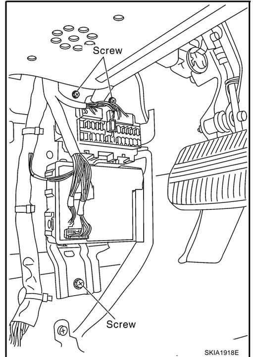
4. Raise the pawl of fuse block and remove bracket from fuse block to remove BCM.
