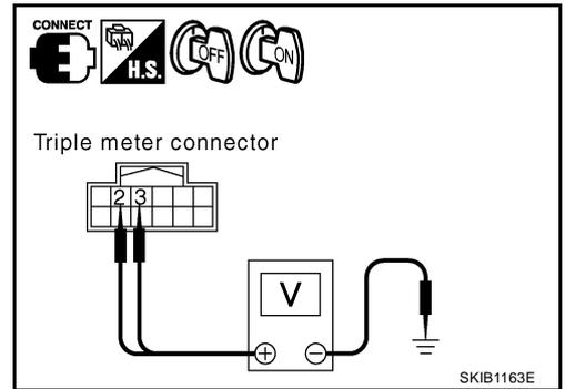
2. Check voltage between unified meter and A/C amp. harness connector terminals and ground.
