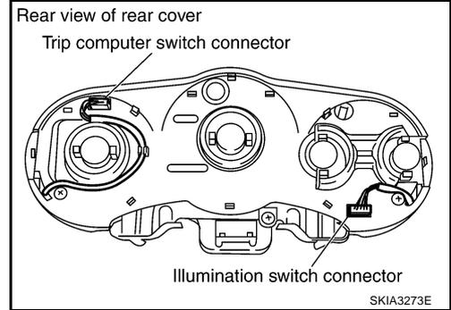
5. Remove screws (2) and remove rear cover.
