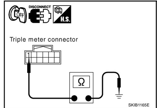
4. Check continuity between unified meter and A/C amp. harness connector M49 terminals 29 (B), 30 (B) and ground.
