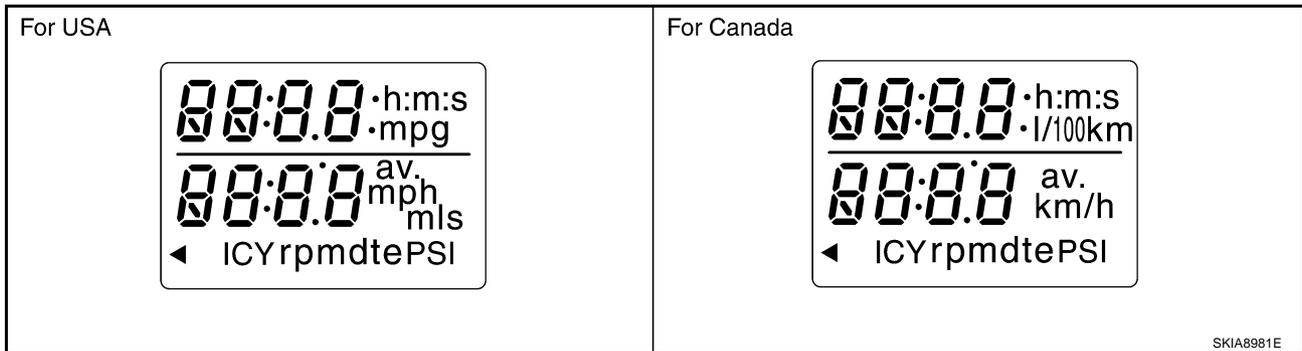
5. Push the odo/trip meter switch. Each meter/gauge should indicate as shown in the figure while pushing odo/trip meter switch.
