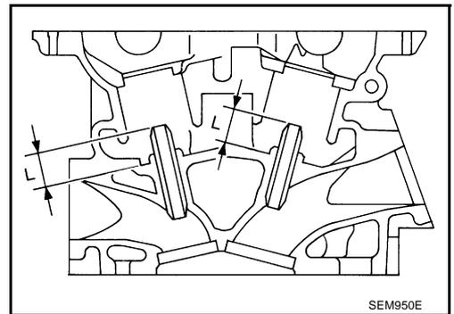
6. Using valve guide reamer (commercial service tool), apply reamer finish to valve guide.
