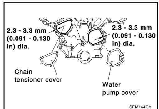
5. Install front timing chain case as follows:
