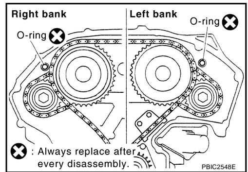
25. Remove water pump cover and chain tensioner cover from front timing chain case.
