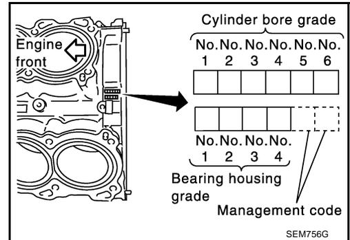
2. "Main Bearing Selection Table" columns correspond to journal diameter grade on front side of crankshaft.
