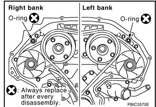
24. Remove water pump cover and chain tensioner cover from front timing chain case.
