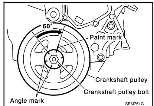
19. Rotate crankshaft pulley in normal direction (clockwise when viewed from engine front) to confirm it turns smoothly.
