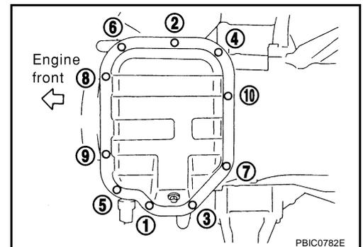
5. Install oil pan drain plug.
