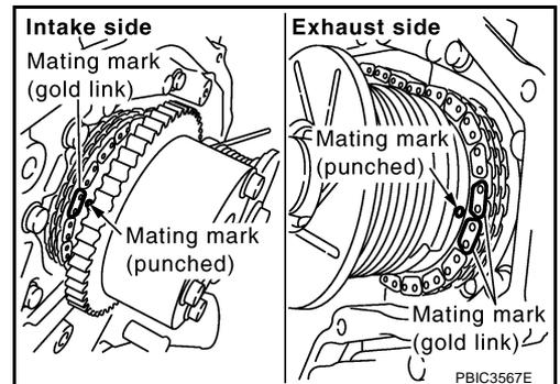
d. Tighten camshaft sprocket mounting bolts.
