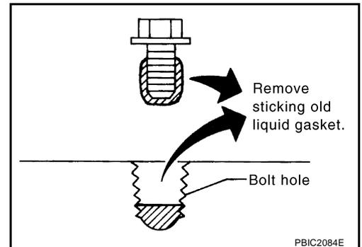
36. Use scraper to remove all traces of liquid gasket from water pump cover, chain tensioner cover and intake valve timing control covers.
