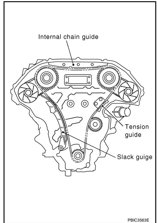
28. Remove timing chain (primary) and crankshaft sprocket.
