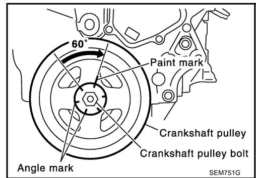
18. Rotate crankshaft pulley in normal direction (clockwise when viewed from engine front) to confirm it turns smoothly.
