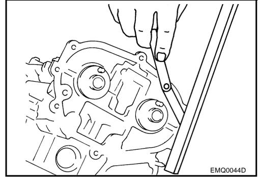
8. Inspect and adjust the valve clearance. Refer to [EM-112, "Valve Clearance"](#) .
