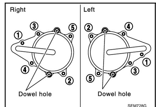
15. Remove left and right valve timing control covers (including magnet retarder and cover) with the following procedure. (For 35<sup>th</sup> Anniversary)
