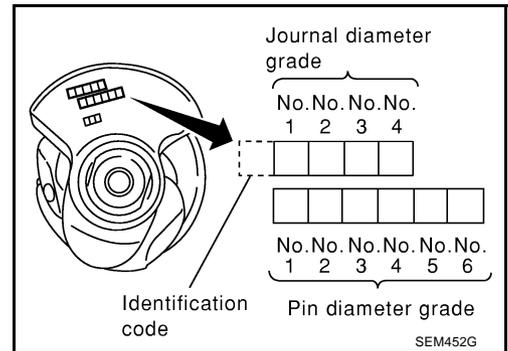
3. Select main bearing grade at the point where selected row and column meet in "Main Bearing Selection Table".
