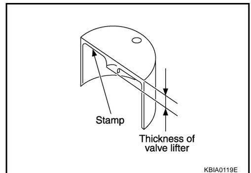
Available thickness of valve lifter: 27 sizes with range 7.88 to 8.40 mm (0.3102 to 0.3307 in) in steps of 0.02 mm (0.0008 in) (when manufactured at factory). Refer to [EM-171, "Available Valve Lifter"](#).
