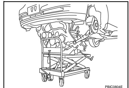
2. Remove rear engine mounting member bolts.
