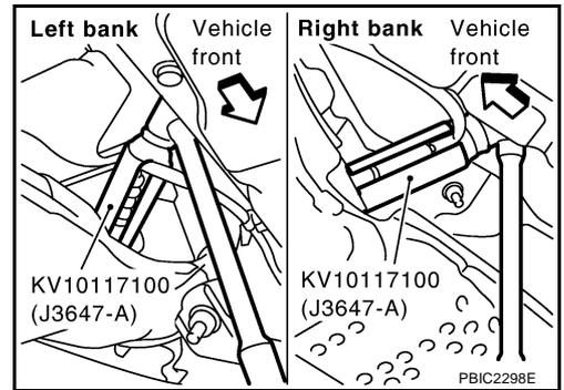
7. Remove exhaust mounting bracket between three way catalysts (right and left bank) and transmission. Refer to [EX-3. "EXHAUST SYSTEM"](#).
