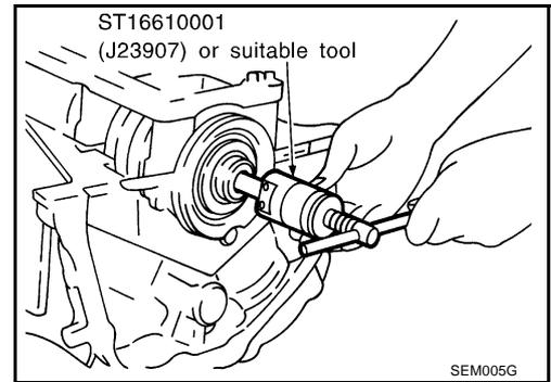
13. Remove rear oil seal retainer.
