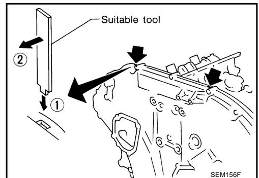
23. Remove O-rings from rear timing chain case.
