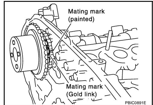
c. After confirming the mating marks are aligned, tighten camshaft sprocket mounting bolts.
