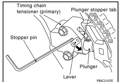
c. Insert plunger into tensioner body by pressing slack guide.
