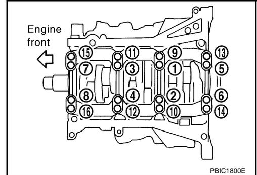
c. Turn all bolts another 90 to 95 degrees clockwise [Target: 90 degrees (Angle tightening)].
