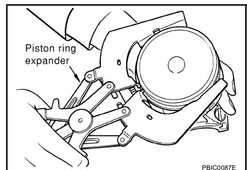
18. Remove piston from connecting rod as follows:
