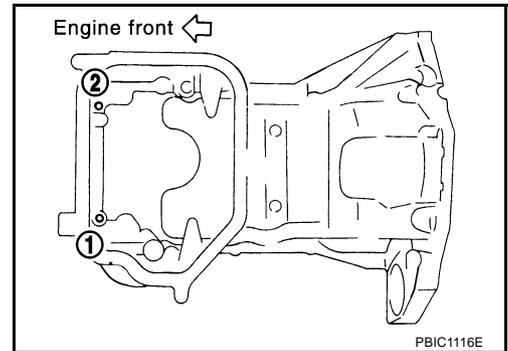
7. Install oil pan (lower). Refer to [EM-28, "OIL PAN AND OIL STRAINER"](#) .
