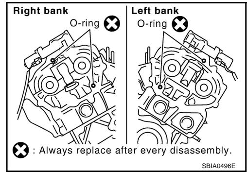
34. Remove O-rings from cylinder block.
