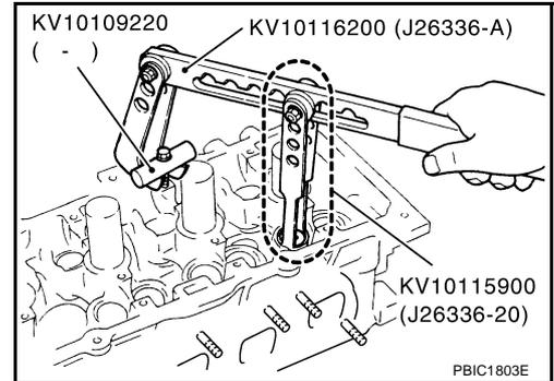
5. Remove valve spring retainer, valve spring and valve spring seat.
