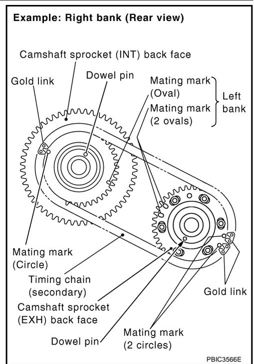
c. Make sure that timing chain (secondary) is not loose from each camshaft sprocket.
