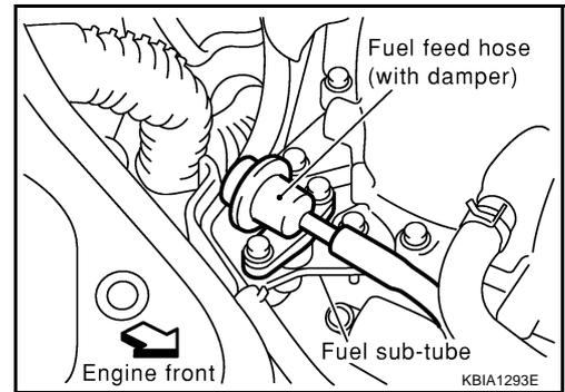
5. When separating fuel feed hose (with damper) and centralized under-floor piping connection, disconnect quick connector as follows:
