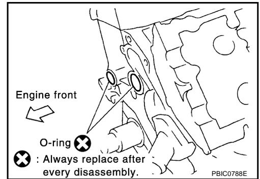
34. Remove timing chain tensioners (secondary) from cylinder head as follows, if necessary.
