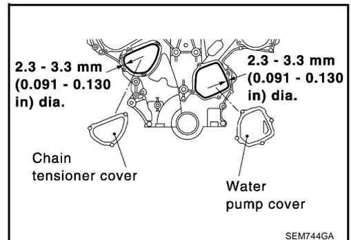
13. Install front timing chain case as follows:
