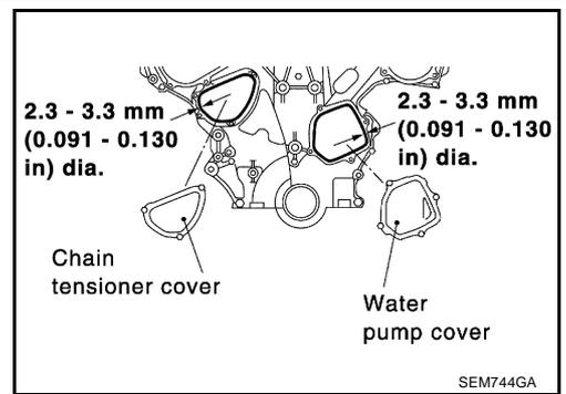
14. Install front timing chain case as follows:
