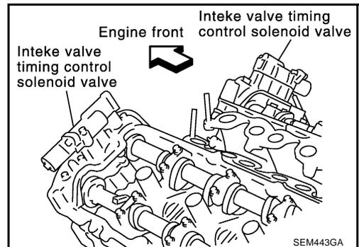
4. Remove intake and exhaust camshaft brackets.
