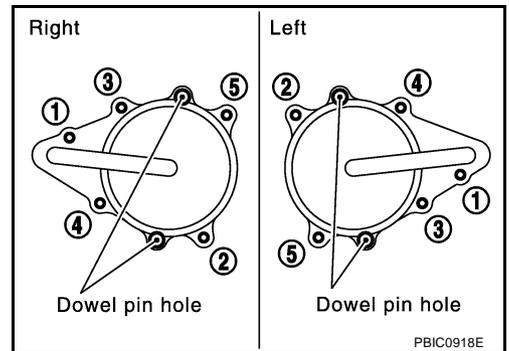
15. Install oil pans (upper and lower). Refer to [EM-28, "OIL PAN AND OIL STRAINER"](#).
