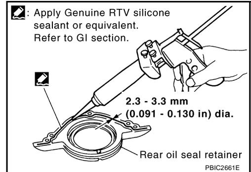
4. Install rear oil seal retainer to cylinder block. Refer to [EM-137, "CYLINDER BLOCK"](#) .
