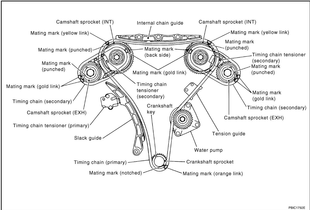
1. Install timing chain tensioners (secondary) to cylinder head as follows if removed. Refer to [EM-106, "INSTALLATION"](#).
