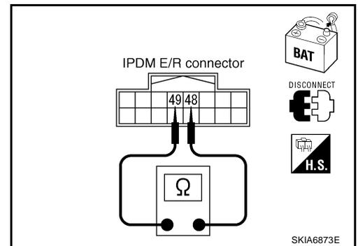
**CAN Communication Circuit Inspection****1. CHECK CONNECTOR**
