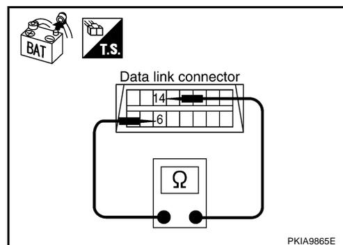
**Unified Meter and A/C Amp. Circuit Inspection****1. CHECK CONNECTOR**
