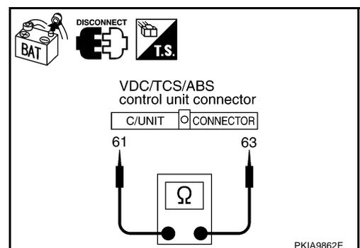
**IPDM E/R Circuit Inspection****1. CHECK CONNECTOR**
