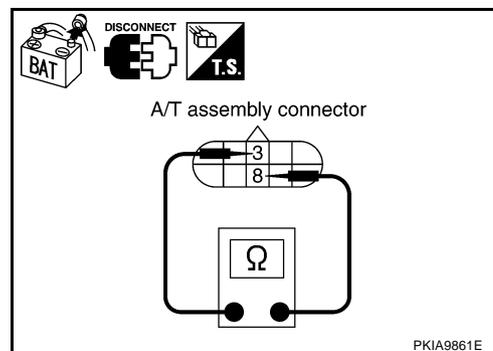
**Data Link Connector Circuit Inspection****1. CHECK CONNECTOR**
