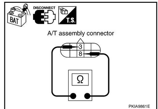
**Data Link Connector Circuit Inspection****1. CHECK CONNECTOR**
