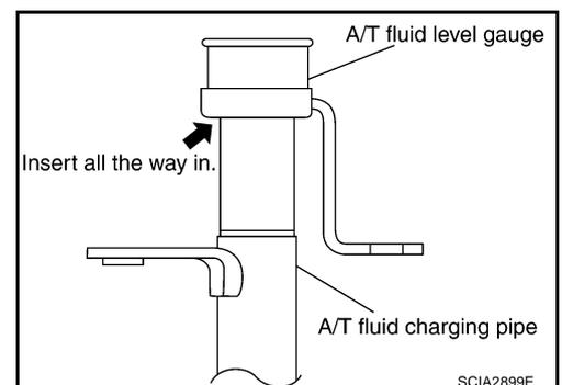
9. Install the removed A/T fluid level gauge in the A/T fluid charging pipe.
