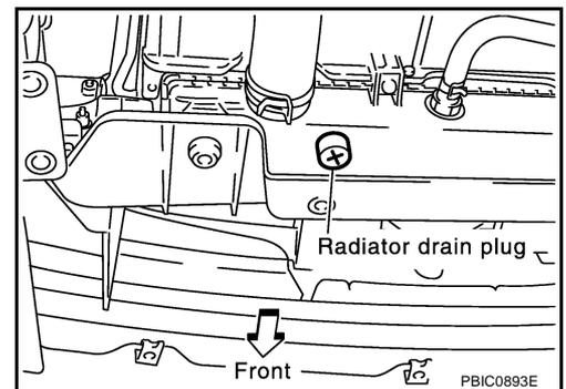
When drain all of engine coolant in the system, open water drain plugs on engine cylinder block. Refer to [EM-139, "DISASSEMBLY"](#).
