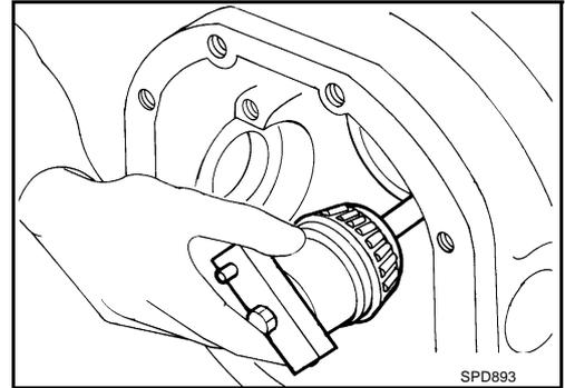
4. Assemble the pinion front bearing inner race and the J-34309-2 gauge anvil. Assemble them together with the J-34309-1 gauge screw in gear carrier. Make sure that the pinion height gauge plate, J-34309-16, will turn a full 360 degrees. Tighten the two sections together by hand.
