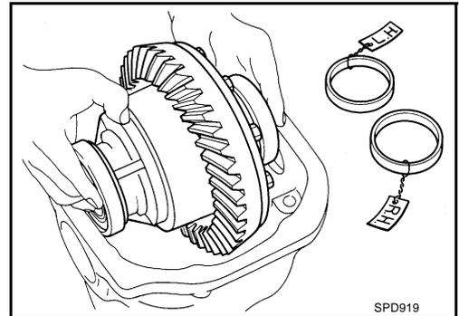
14. Insert selected left and right side bearing adjusting washers in place between side bearings and gear carrier.
