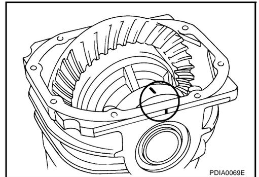
6. Measure the turning torque of the carrier at the drive gear mounting bolts with a spring gauge.
