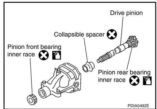
7. Using suitable spacer, press the pinion front bearing inner race to drive pinion as far as drive pinion nut can be tightened.
