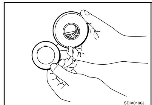
2. Install side gear and thrust washer into differential case B.
