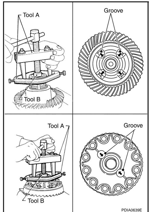
10. For proper reinstallation, paint matching mark on one differential case assembly.
