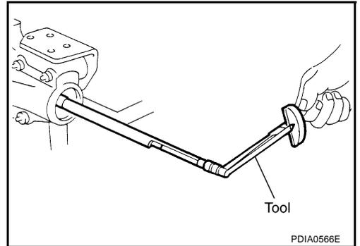
7. Place the J-34309-11 "R200A" pinion height adapter onto the gauge plate and tighten it by hand.
