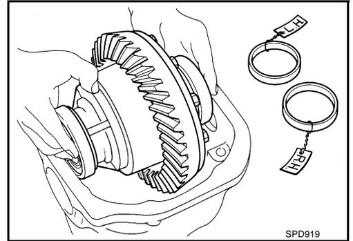
3. Insert left and right original side bearing adjusting washers in place between side bearings and gear carrier.
