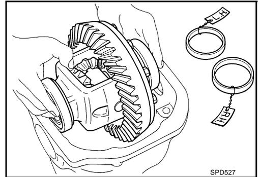
9. Remove side bearing inner race.
