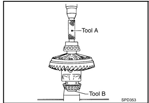
12. Install differential case assembly with side bearing outer races into gear carrier.
