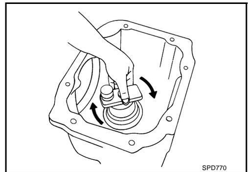
6. Measure the turning torque at the end of the J-34309-2 gauge anvil using preload gauge.
