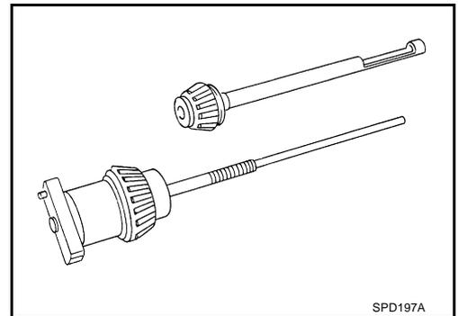
3. Install the pinion rear bearing inner race into gear carrier. Then place the pinion preload shim selector tool, J-34309-1, gauge screw assembly.
