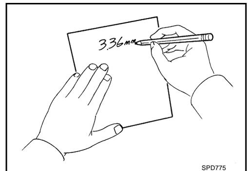
11. Correct the pinion height washer size by referring to the "pinion head number".
