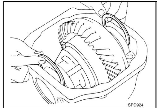
15. Align matching mark on bearing cap with that on gear carrier.
