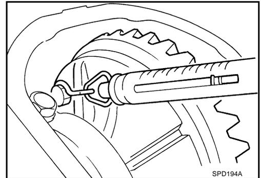
7. If the turning torque is outside the specification, use a thicker/thinner side bearing adjusting washer to adjust. Refer to [RFD-57, "Side Bearing Adjusting Washer"](#).
