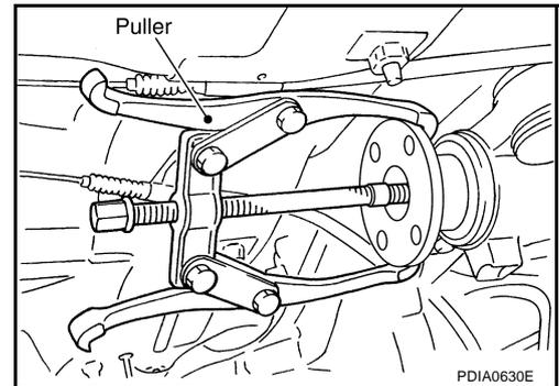
5. Remove front oil seal using the puller.
