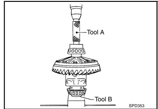
11. Install differential case assembly with side bearing outer races into gear carrier.
