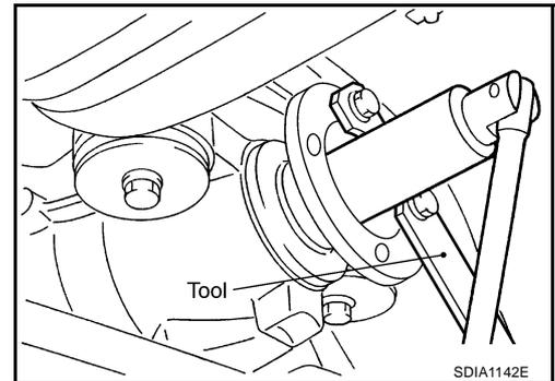
4. Remove companion flange using a puller.
