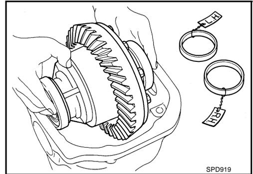
9. Remove side bearing inner race.
