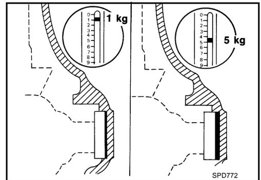
8. Record the total amount of washer thickness required for the correct carrier side bearing preload.
