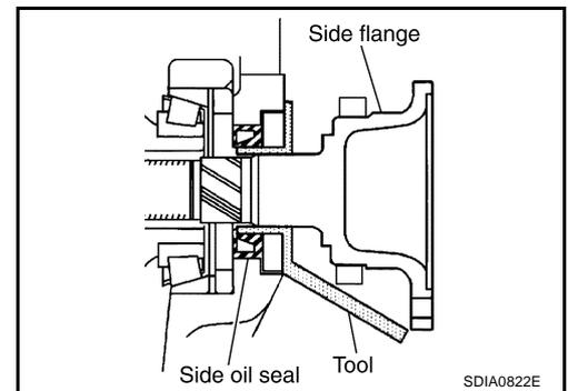
c. Put a suitable drift on the center of side flange, then drive it until sound changes.
