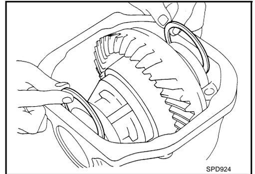
4. Install bearing caps in their correct locations and tighten bearing cap mounting bolts to the specified torque. Refer to [RFD-36. "COMPONENTS"](#).
