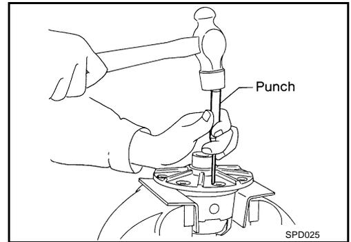
14. Remove pinion mate shaft.
