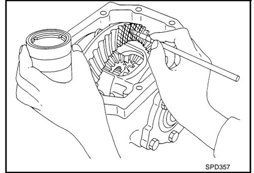
3. Rotate drive gear back and forth several times, check drive pinion gear to drive gear tooth contact.
