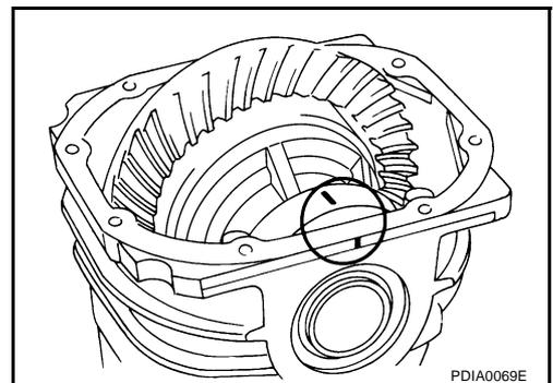
17. Using the drift, drive side oil seals until it becomes flush with the case end.
