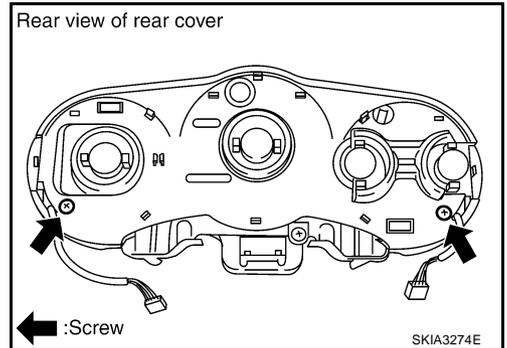
6. Disengage tabs (4) to separate upper cover from rear cover.
