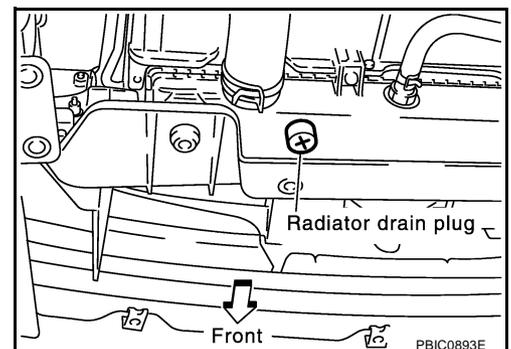
When drain all of engine coolant in the system, open water drain plugs on engine cylinder block. Refer to [EM-138, "DISASSEMBLY"](#).
