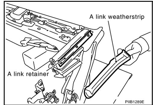
11. Peel a link sealing out.
