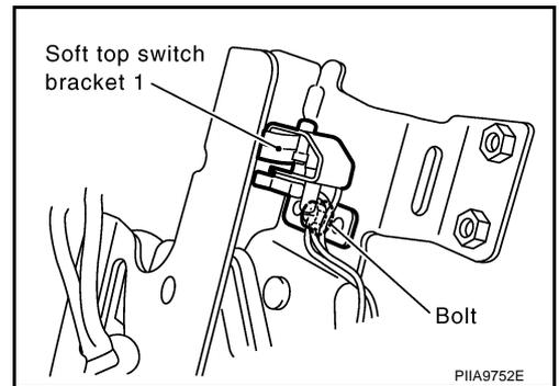
5. Remove limit switches with soft top switch bracket 2 by removing bolt.
