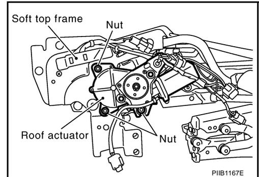
3. Disconnect soft top actuator harness connector.
