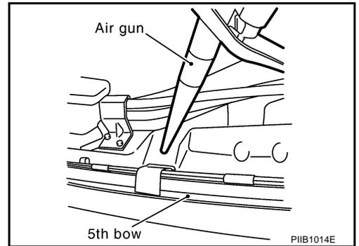
2. Remove the remains drawn to both ends by the air blow from the gap.
