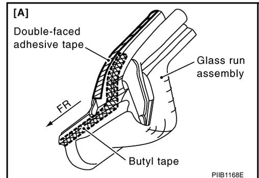
Water may be entering through connection between front pillar and front edge of soft top.
