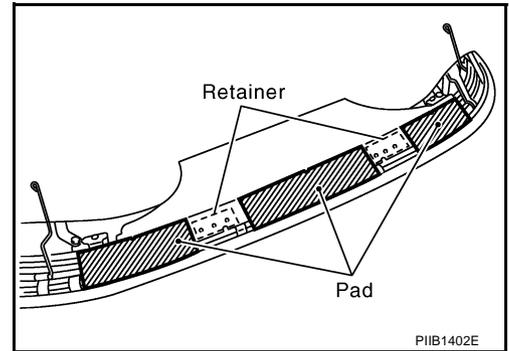
2. Remove screws, and then remove 5th bow side finisher (RH/LH).
