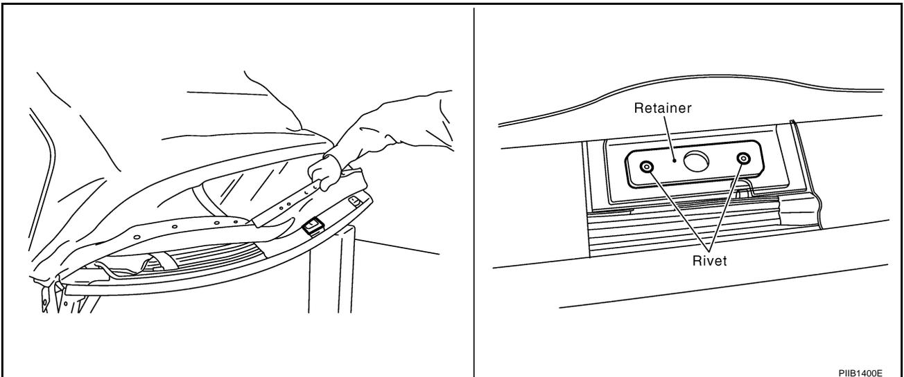
28. Pull up cover from the bottom of C link.
