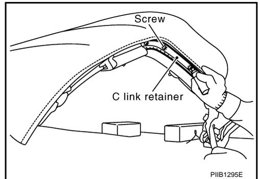
20. Remove clips on the bottom edge of C link and 5th bow weatherstrip.
