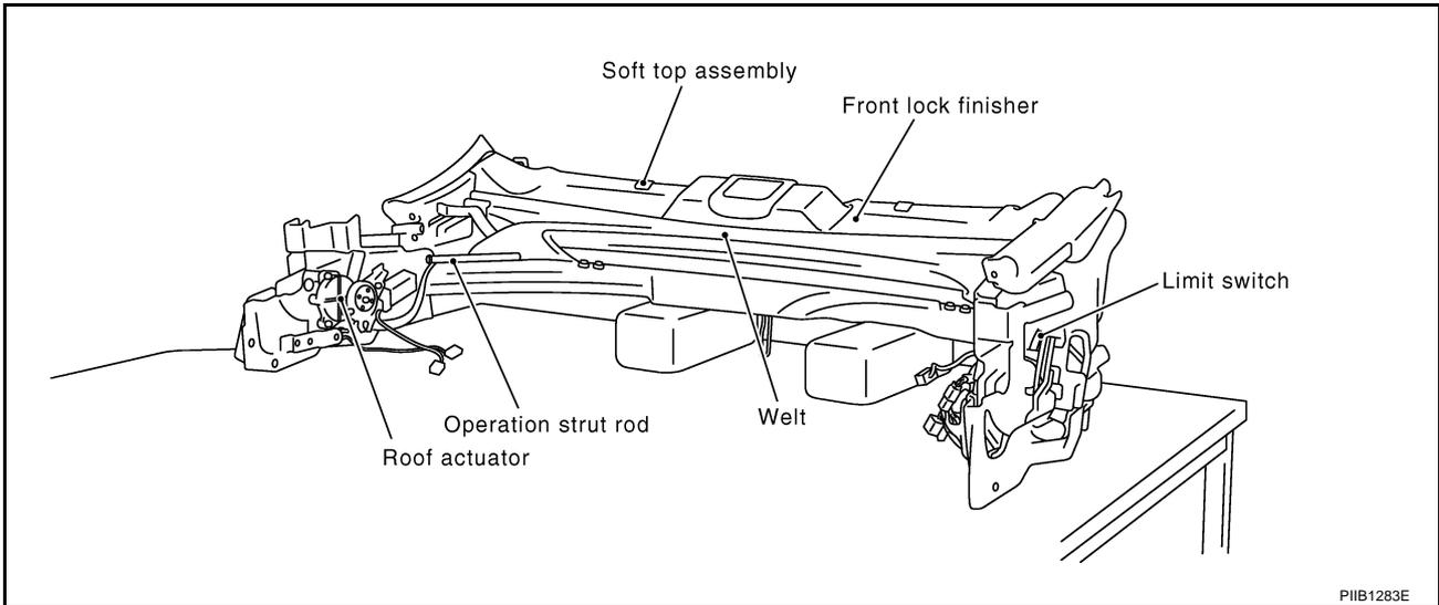
3. Remove roof actuator (RH/LH). Refer to [RF-108, "Removal and Installation of Roof Actuator"](#).
