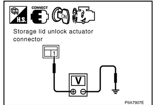
**2. CHECK STORAGE LID UNLOCK ACTUATOR CIRCUIT**
