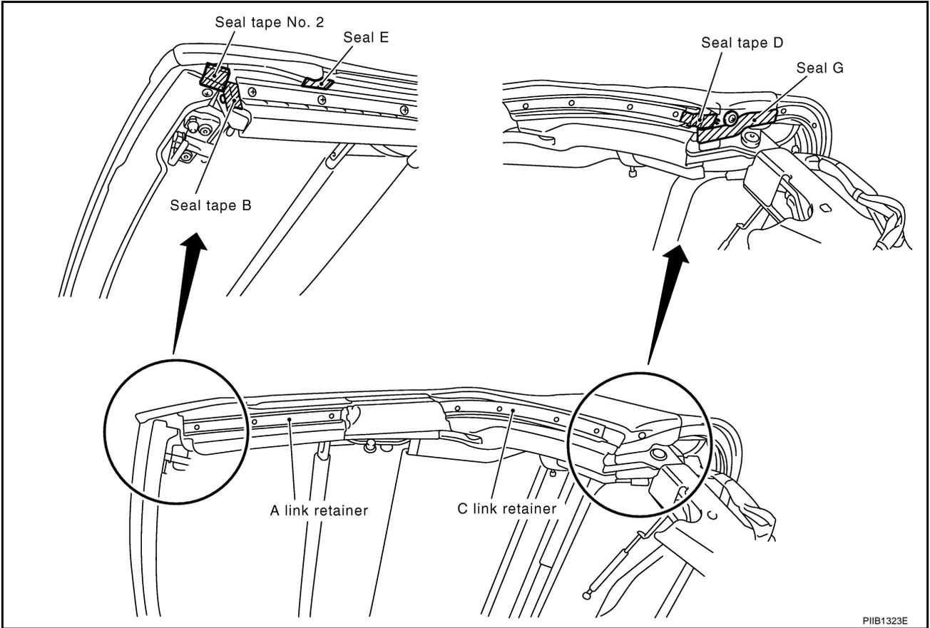
26. Install C link and 5th bow weather strip to 5th bow and C link.
