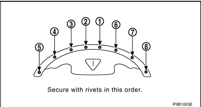
18. Secure soft top cover to C link with rivet.
