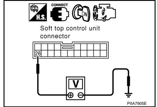
**Check Storage Lid Unlock Actuator (Open Operate)**
