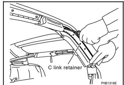
22. Apply seal to C link lower installation position.
