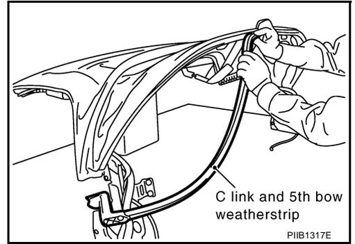
22. Remove screws, and then remove 5th bow retainer.
