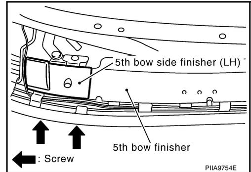
15. Remove 5th bow finisher by pulling the finisher up.
