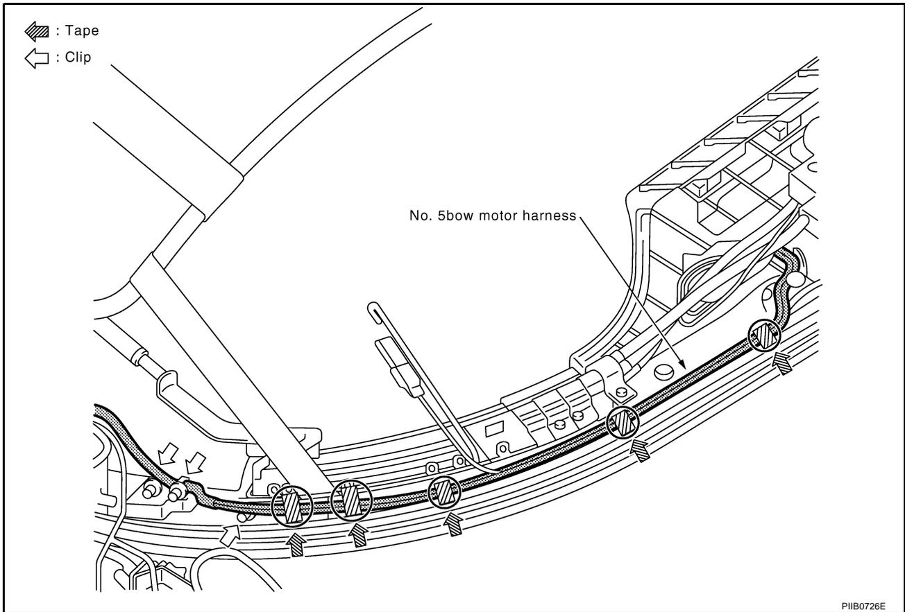
4. Replace rivet retainer on back of 5th bow finisher with a new one.
