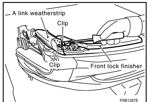
9. Pull up front lock lever, and then disengage clips to remove front lock finisher.
