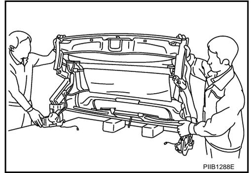
6. Protect the limit switch contact around the rotation axis of the 5th bow on the left side of soft top with tape.
