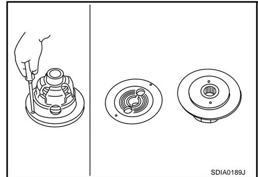
15. Separate differential case A and B, then remove viscous coupling, pinion mate gear, pinion mate thrust washer, side gear and side gear thrust washer from differential cases.
