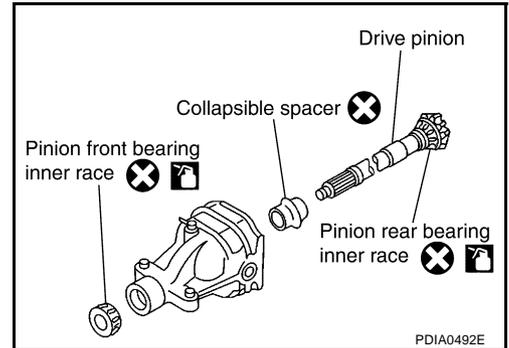
7. Using suitable spacer, press the pinion front bearing inner race to drive pinion as far as drive pinion nut can be tightened.
