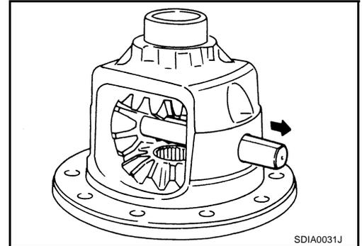
15. Turn pinion mate gear, then remove pinion mate gear, pinion mate thrust washer, side gear and side gear thrust washer from differential case.
