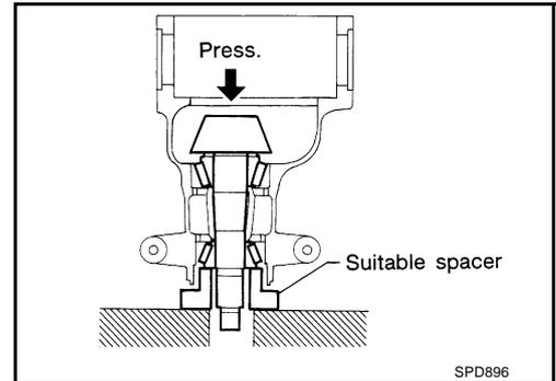
8. Using the drift, install front oil seal as shown in the figure.
