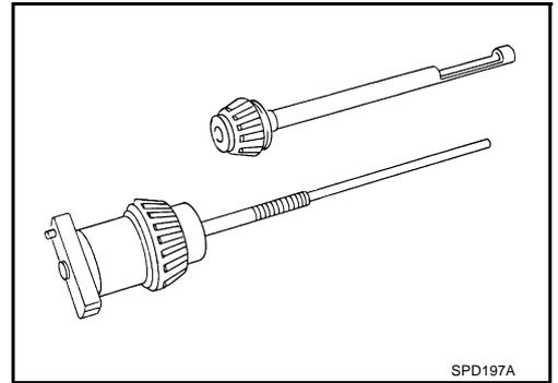
3. Install the pinion rear bearing inner race into gear carrier. Then place the pinion preload shim selector tool, J-34309-1, gauge screw assembly.
