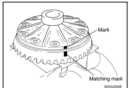
8. Apply thread locking sealant into the thread hole of drive gear.
