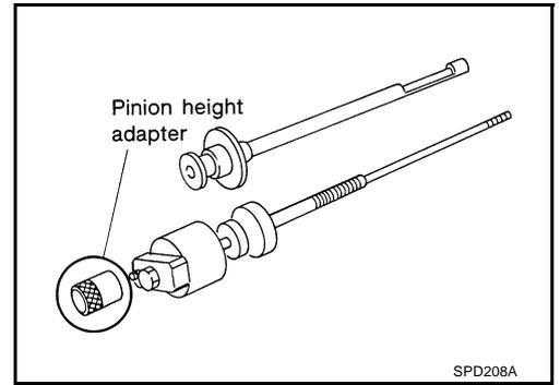
8. Position the side bearing discs, J-25269-4, and arbor firmly into the side bearing bores. Install the bearing caps and tighten bearing cap mounting bolts to the specified torque. Refer to [RFD-19, "COMPONENTS"](#).
