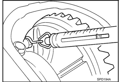
7. If the turning torque is outside the specification, use a thicker/thinner side bearing adjusting washer to adjust. Refer to [RFD-60, "Side Gear Thrust Washer"](#).
