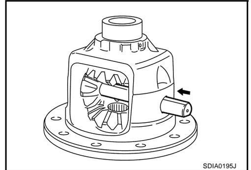
6. Drive a lock pin into pinion mate shaft, using a punch. Make sure lock pin is flush with differential case.
