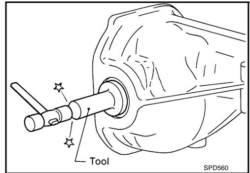
17. Check and adjust drive gear runout, tooth contact, drive gear to drive pinion backlash, and total preload torque. Refer to [RFD-20, "Drive Gear Runout"](#) , [RFD-21, "Tooth Contact"](#) , [RFD-22, "Backlash"](#) and [RFD-20, "Total Preload Torque"](#) .
