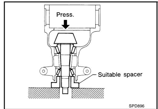
8. Using the drift, install front oil seal as shown in the figure.
