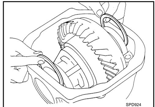
4. Install bearing caps in their correct locations and tighten bearing cap mounting bolts to the specified torque. Refer to [RFD-55, "Differential Assembly"](#).
