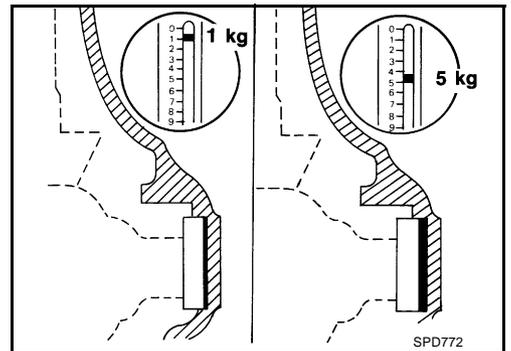
8. Record the total amount of washer thickness required for the correct carrier side bearing preload.
