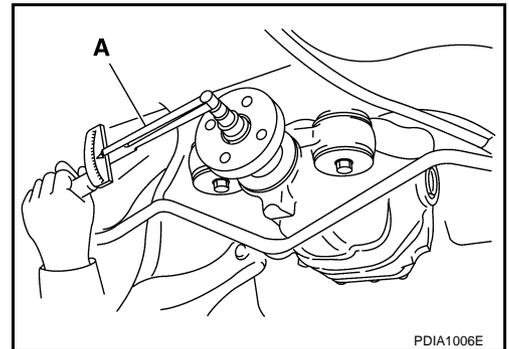
8. Remove drive pinion lock nut using the flange wrench.
