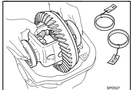
13. Insert selected left and right side bearing adjusting washers in place between side bearings and gear carrier.
