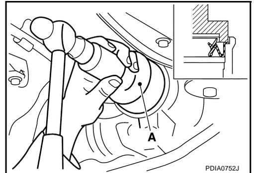
3. Align the matching mark of drive pinion with the matching mark of companion flange, and then install the companion flange.
