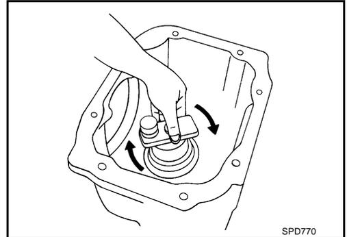
6. Measure the turning torque at the end of the J-34309-2 gauge anvil using preload gauge.
