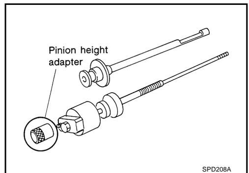
8. Position the side bearing discs, J-25269-4, and arbor firmly into the side bearing bores. Install the bearing caps and tighten bearing cap mounting bolts to the specified torque. Refer to [RFD-39, "COMPONENTS"](#).
