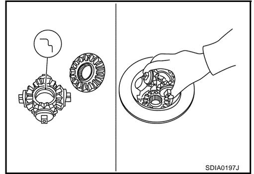
4. Install viscous coupling into differential case B.
