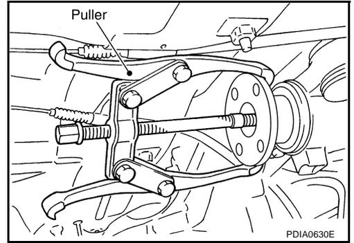
11. Remove front oil seal using the puller.
