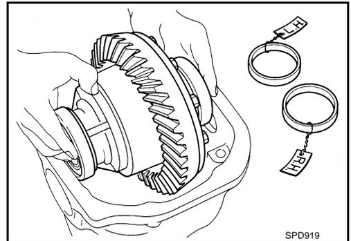
3. Insert left and right original side bearing adjusting washers in place between side bearings and gear carrier.
