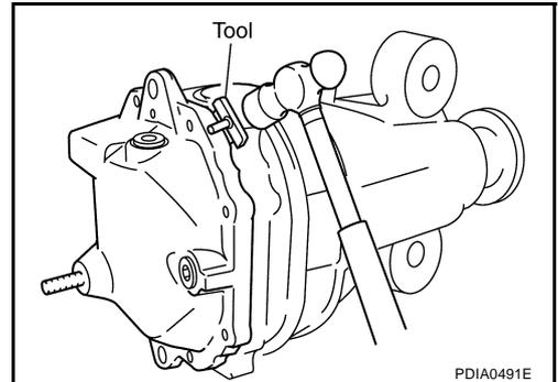
5. Using two 45 mm (1.77 in) spacers, mount carrier on the attachment.
