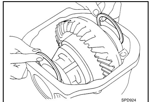
15. Align matching marks on bearing cap with that on gear carrier.
