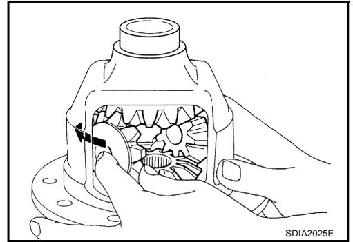
4. Align the lock pin holes on differential case with shaft, and install pinion mate shaft.
