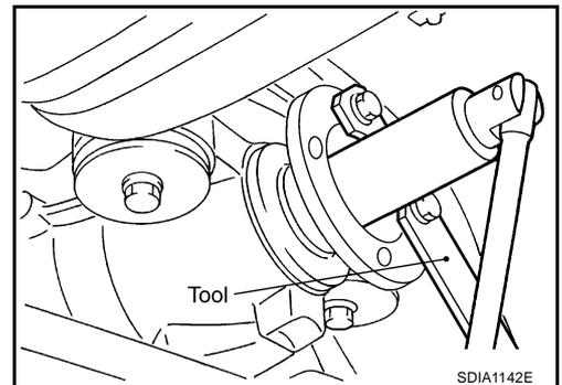
9. Put matching mark on the end of the drive pinion. The matching mark should be in line with the matching mark A on companion flange.
