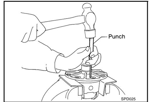
14. Remove pinion mate shaft.
