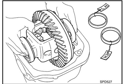
9. Remove side bearing inner race.
