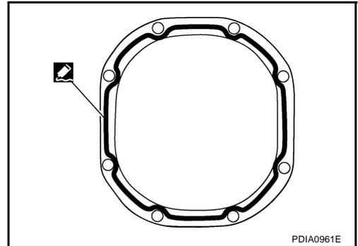
20. Install rear cover on gear carrier and tighten mounting bolts with the specified torque. Refer to [RFD-39, "COMPONENTS"](#).
