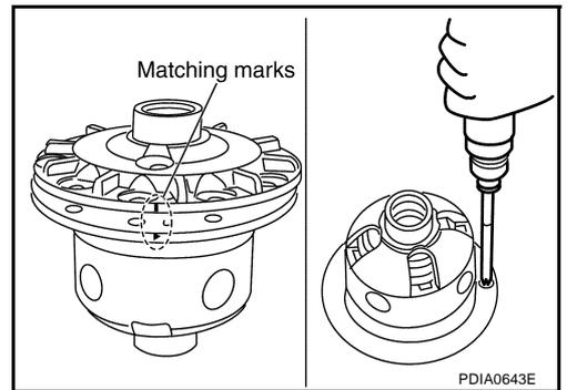
8. Align the matching mark of differential case with the mark of drive gear, then place drive gear.
