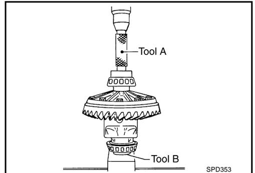
11. Install differential case assembly with side bearing outer races into gear carrier.
