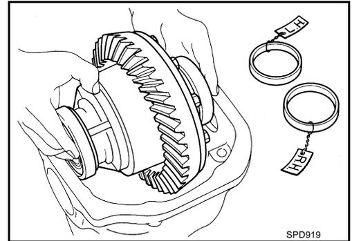
9. Remove side bearing inner race.
