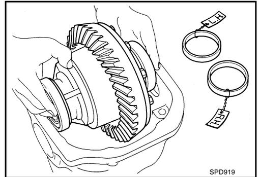
14. Insert selected left and right side bearing adjusting washers in place between side bearings and gear carrier.
