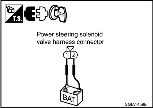
**7. CHECK VEHICLE SPEED SIGNAL CIRCUIT**
