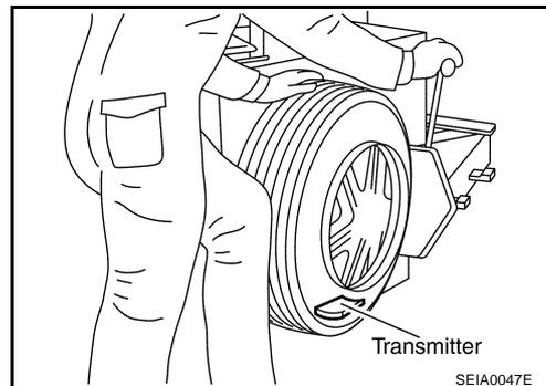
3. Turn tire so that valve hole is at bottom and bounce so that transmitter is near valve hole. Carefully lift tire onto turntable and position valve hole (and transmitter) 270 degree from mounting/dismounting head.
