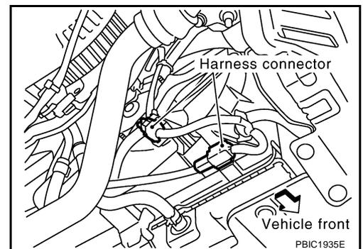
7. Remove mounting bolts to lift up and radiator cooling fan assembly.
