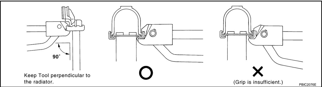
● Use pliers in the locations where radiator plate pliers A [SST: KV99103510 ( — )] cannot be used.
