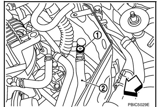
3. Fill radiator with water until water spills from the air relief hole, then close air relief plug. Fill radiator and reservoir tank with water and reinstall radiator cap.
