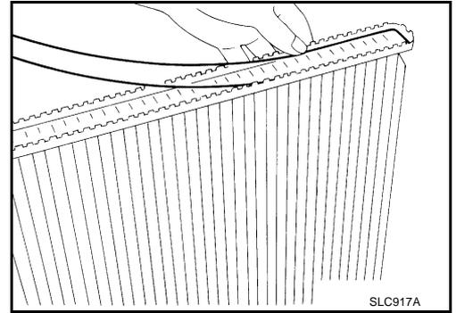
3. Caulk tank in numerical order as shown in the figure with radiator plate pliers A (SST).
