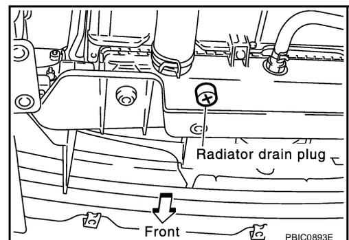
When drain all of engine coolant in the system, open water drain plugs on engine cylinder block. Refer to [EM-108, "DISASSEMBLY"](#) .
