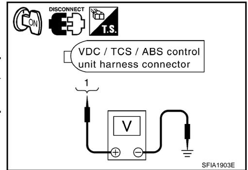
3. Check continuity between VDC/TCS/ABS control unit and ground.
