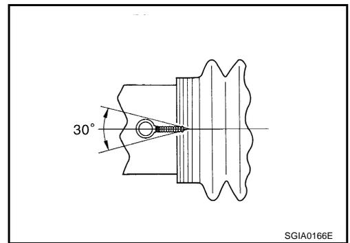
22. Install cylinder tubes to gear housing assembly.
