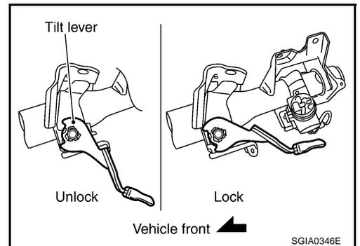
2. When tilt lever is in the locked position (operation range is about 40°), tighten lock nut at the specified torque to make tilt lever locked.
