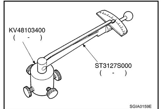
15. Measure pinion rotating torque with torque adapter (SST) and preload gauge (SST), then confirm whether its reading is within the specified value. If the reading is not within the specified value, readjust screw angle with adjusting screw. Change gear assembly to new one, if the reading is still not within the specified value or the rotating torque of adjusting screw is less than 5 N·m (0.51kg·m, 44 in·lb)
