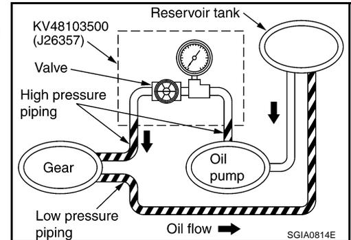
2. Start engine. Allow engine to run until tank temperature reaches 50 to 80°C (122 to 176°F).
