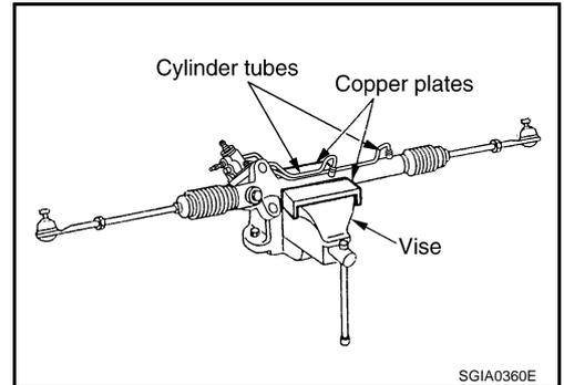
23. Tighten lightly inner socket in specified length "L", then tighten lock nut at specified torque. Refer to [PS-19, "COMPONENTS"](#). Reconfirm if inner socket length is within limit of specified length "L".
