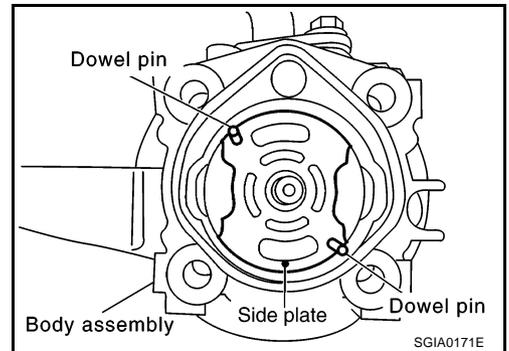
5. Install cam ring on side plate as follows;
