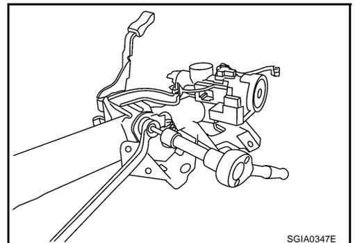
**Tightening torque : 25 - 34 N·m (2.6 - 3.4 kg·m, 19 - 25 ft·lb)**
