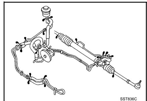
4. If fluid leakage at connections is noticed, then loosen flare nut and then retighten. Do not over tighten connector as this can damage O-ring, washer and connector.
