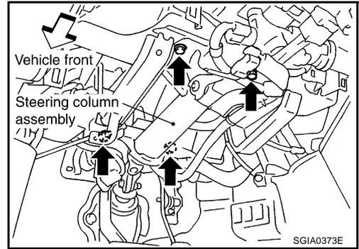
16. Raise vehicle, then loosen bolt for lower yoke of lower joint and remove joint together with lower shaft.
