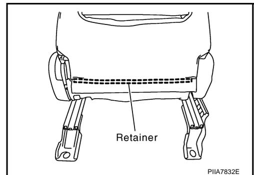
10. After removing the seatback trim and pad, remove the hog rings to separate the trim and pad.
