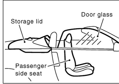
1. Passenger seatback tilts forward by approximately 6° as soon as windows go down, when soft top switch has been pushed on CLOSE.
