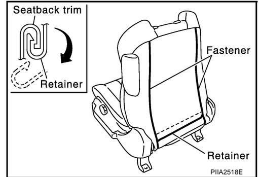
2. Remove the stay securing the inner cloth.
