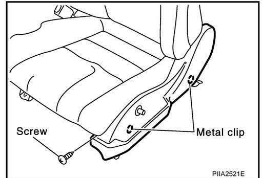
4. Remove bolts on the under side of seat cushion.
