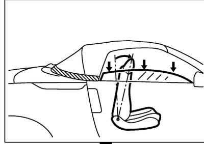
2. Soft top OPEN operation starts as soon as the passenger seatback tilt forward operation completes.
