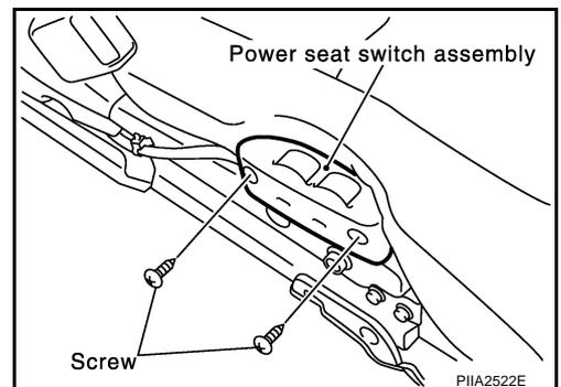
Insert a screwdriver in lower side of power seat switch and remove it (passenger seat for coupe).
