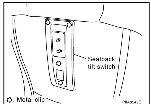
2. Disconnect seatback tilt switch harness connector.
