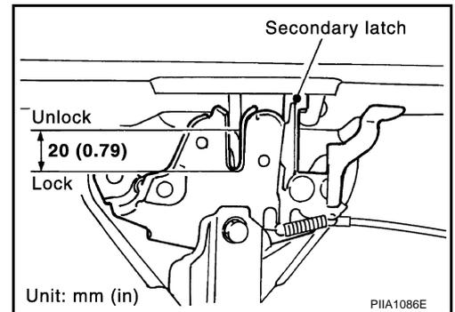
3. Check the hood lock lubrication condition. If necessary, apply "body grease" to the points shown in the figure.
