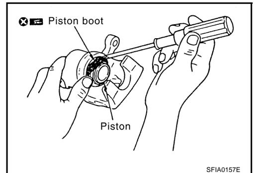
3. Apply brake fluid or rubber grease to piston, insert into cylinder body by hand and firmly attach the piston boot piston-side lip into the piston groove.
