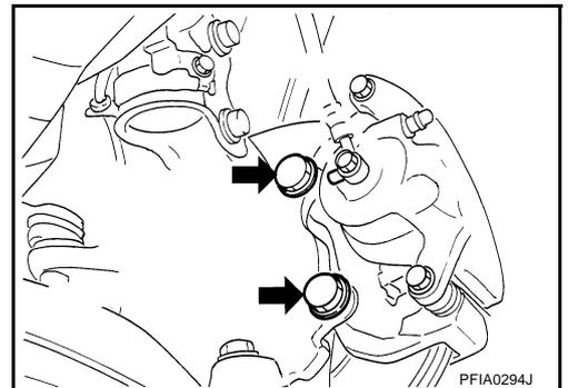
3. Install brake hose to caliper assembly, and tighten union bolts to the specified torque.
