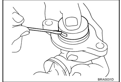
2. Attach attachment in inner kit to reservoir cap as shown in the figure.
