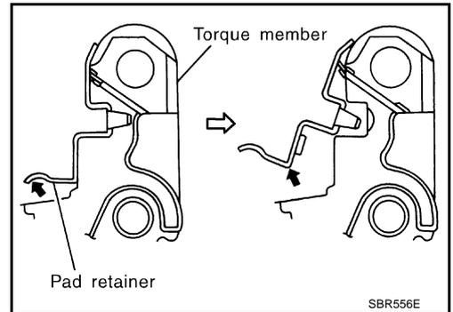
2. Remove sliding pins and sliding pin boots from torque member.
