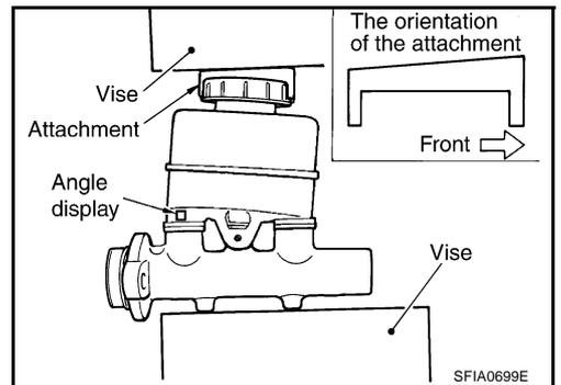
4. Using a pin punch [commercial service tool: diameter Approx. 4 mm (0.16 in)], remove mounting pins on the reservoir tank.
