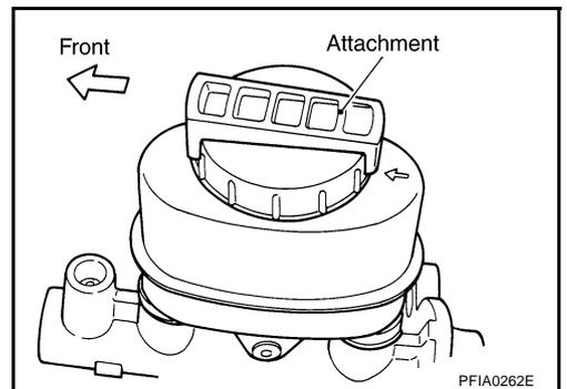
3. Place the side of the cylinder body with chamfering around the pin insertion hole facing up, and secure master cylinder assembly with a vise.
