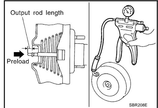
Standard dimension when vacuum  $-66.7 \text{ kPa}$  ( $-500 \text{ mmHg}$ ,  $-19.69 \text{ inHg}$ ) :  $10.4 \text{ mm}$  (  $0.409 \text{ in}$  )
