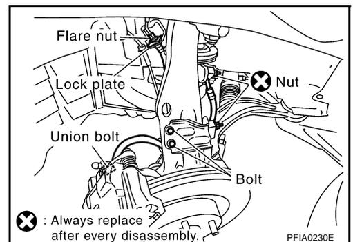
4. Refill new brake fluid and bleed air. Refer to [BR-10, "Bleeding Brake System"](#).
