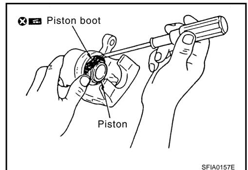
3. Apply a brake fluid to piston, insert into cylinder body by hand and firmly attach the piston boot piston-side lip into the piston groove.
