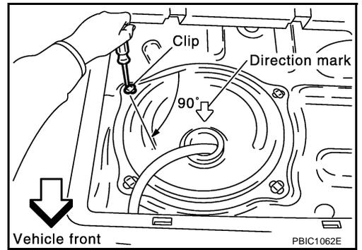
7. Disconnect harness connector and fuel feed tube.
