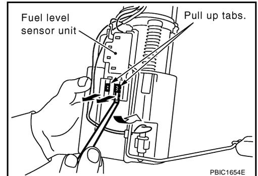
3. After fixing tabs are disengaged, slide fuel level sensor unit out in direction shown by the arrow.
