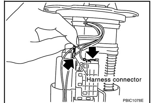
2. Using a suitable tool, pull up tabs points shown in the figure (2 points) to release the tabs, and disconnect them.
