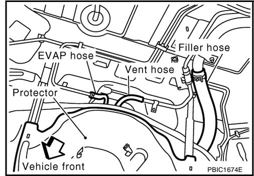
9. Remove fuel tank mounting band bolts while supporting fuel tank.
