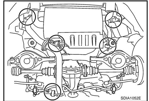
2. Attach protector (special service tool) to propeller shaft.
