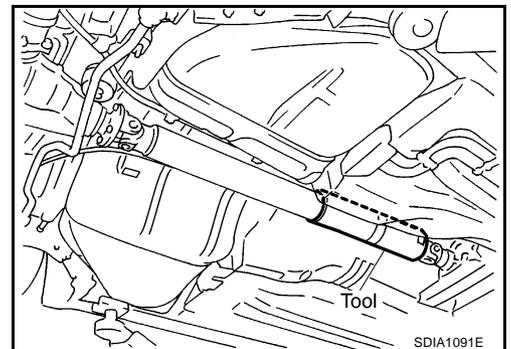
3. Put matchmarks on flanges and separate propeller shaft from final drive.
