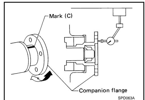
6. Position companion flange and propeller shaft using alignment marks A and B. Set the marks A and B as close to each other as possible. Temporarily attach bolts and nuts.
