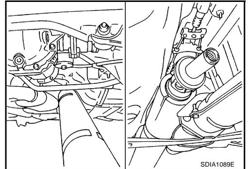
3. Face mark C on final drive joint upward.
