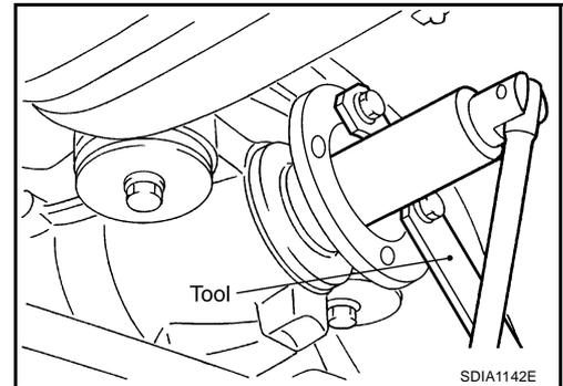
4. Using the puller, remove the companion flange.
