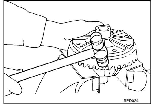
4. Drive out pinion mate shaft lock pin with punch from drive gear side.
