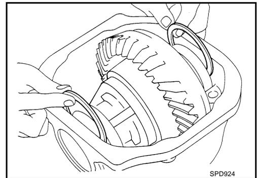
4. Install the bearing caps in their correct locations and torque the bearing cap retaining bolts.
