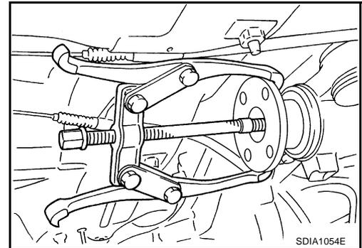
5. Using the oil seal puller, remove front oil seal.
