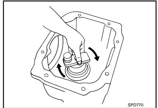
6. Measure the turning torque at the end of the J34309-2 gauge anvil using torque wrench J-25765A.
