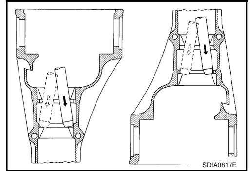
9. Remove pinion rear bearing inner race and drive pinion height adjusting washer with Tool.
