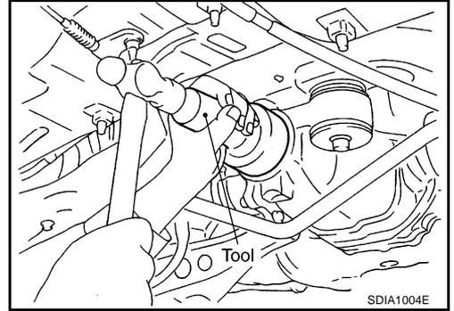
2. Align the matching mark of drive pinion with the matching mark B of companion flange, then install the companion flange.
