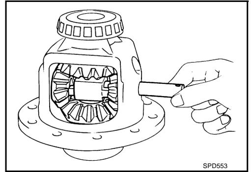
3. Adjust clearance between rear face of side gear and thrust washer by selecting side gear thrust washer. Refer to [RFD-34, "AVAILABLE SIDE GEAR THRUST WASHERS"](#). Use two feeler gauges to prevent leaning of side gear as shown, figure.
