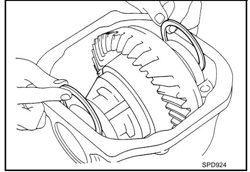
4. Align mark on bearing cap with that on gear carrier and install bearing cap on gear carrier.
