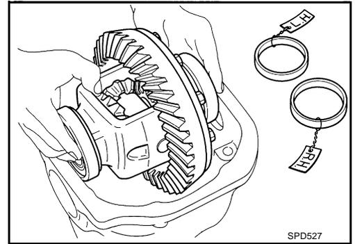
3. Insert left and right side bearing adjusting washer in place between side bearings and gear carrier.
