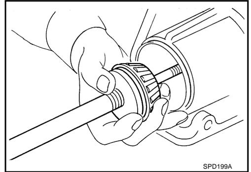
5. Turn the assembly several times to seat the bearings.
