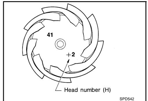
There are two numbers painted on the drive pinion gear. The first one refers to the drive pinion and drive gear as a matched set. This number should be the same as the number on the drive gear. The second number is the "pinion head height number". It refers to the ideal pinion height from standard for quietest operation. Use the following chart to determine the correct pinion height washer.
