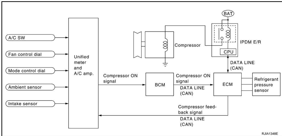
When A/C switch is pressed, turn fan control dial to ON or set mode control dial to D/F, D/F2 or DEF position, unified meter and A/C amp. transmits compressor ON signal to BCM.
