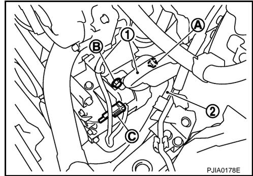
9. Remove mounting bolts (A) from compressor, using power tools.
