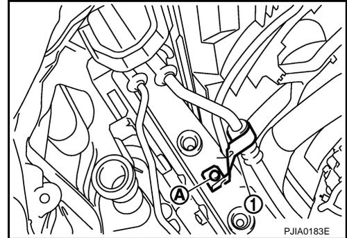
6. Disconnect one-touch joint between high-pressure flexible hose (1) and condenser with disconnecter (SST: 9253089912) (A).
