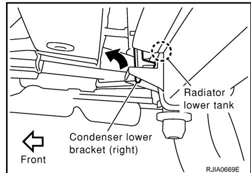
14. Pull condenser forward at an angle. Remove condenser from radiator.
