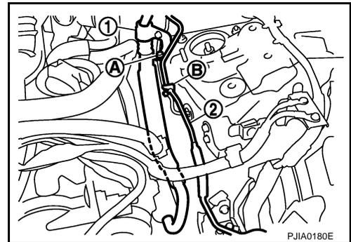
7. Disconnect one-touch joint between low-pressure pipe 1 (1) and low-pressure pipe 2 (2) with disconnecter (SST: 9253089916) (A).
