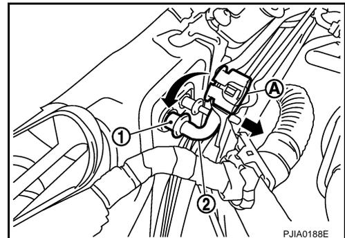
10. Remove mounting nut (A) from low-pressure flexible hose (1). (Compressor side)
