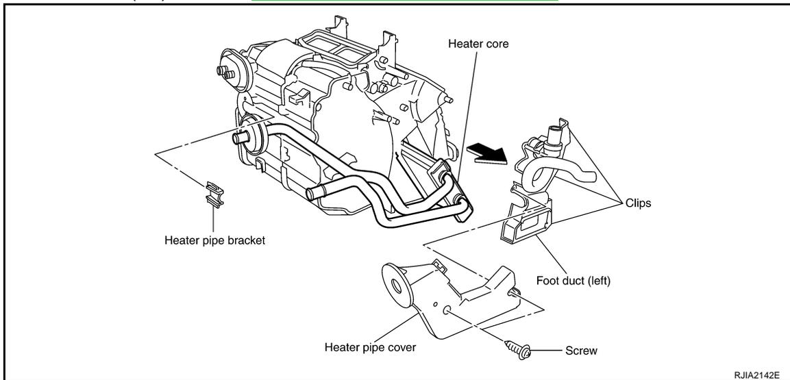
3. Remove mounting screws, and then remove heater pipe cover.
