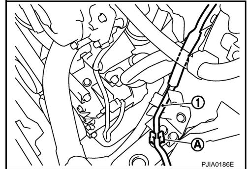
3. Disconnect one-touch joint between high-pressure pipe 1 (1) and condenser with disconnecter (SST: 9253089908) (A).
