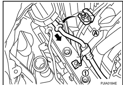
7. Remove mounting nut (A) from high-pressure flexible hose (1), and then remove high-pressure flexible hose.
