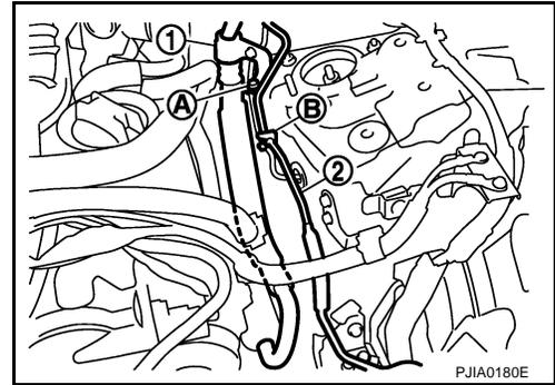
8. Disconnect one-touch joint between low-pressure flexible hose (1) and low-pressure pipe 2 (2) with disconnecter (SST: 9253089916) (A).
