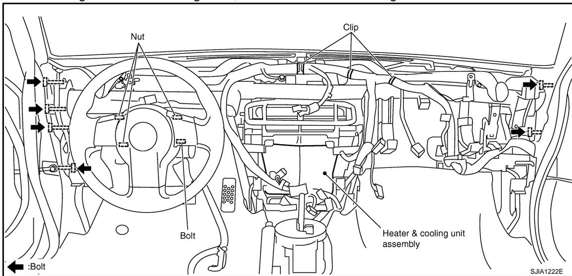
15. Remove heater & cooling unit assembly.
