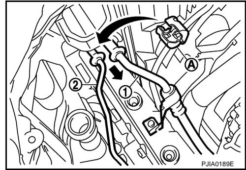
11. Remove radiator upper mount, move radiator and condenser to the engine side.
