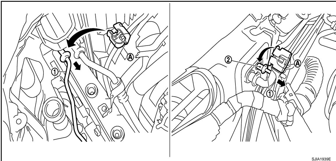
4. Disconnect one-touch joint between high-pressure pipe 1 (1) and high-pressure pipe 2 (2) with disconnecter (SST: 9253089908) (A).
