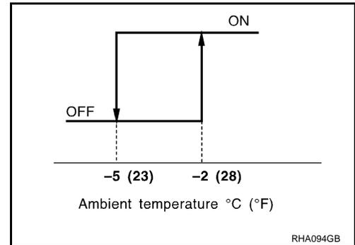
When intake air temperature is higher than  $1^{\circ}\text{C}$  ( $34^{\circ}\text{F}$ ), the compressor turns ON. The compressor turns OFF when intake air temperature is lower than  $-5^{\circ}\text{C}$  ( $23^{\circ}\text{F}$ ).
