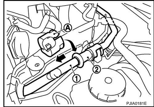
9. Disconnect one-touch joint between low-pressure pipe 1 (1) and low-pressure pipe 2 (2) with disconnecter (SST: 9253089916) (A).
