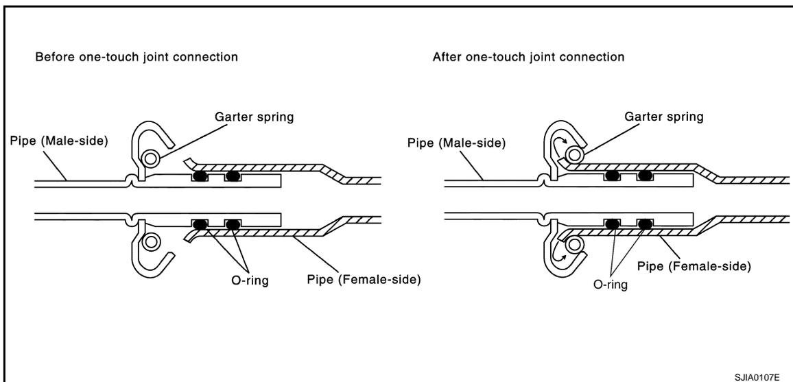
1. Clean piping connection points, and insert male-side piping into female-side piping.
