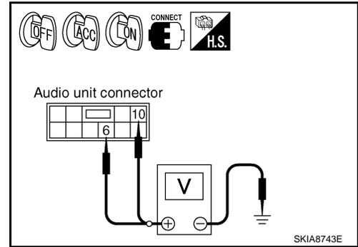
2. Check voltage between BOSE speaker amp., woofer amp. harness connector terminals and ground (BOSE system).
