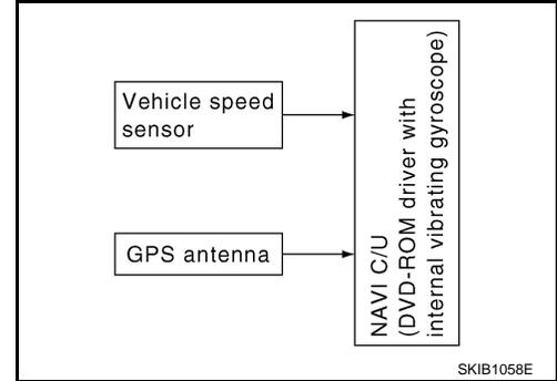
The current vehicle position will be calculated by detecting the distance the vehicle moved from the previous calculation point and its direction.
