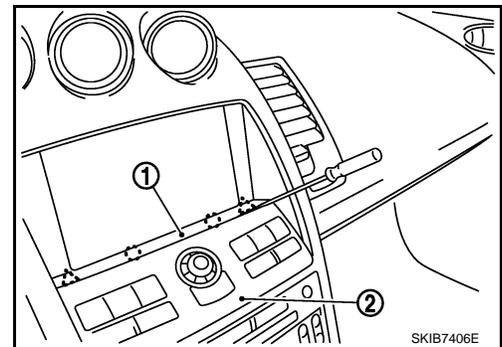
2. Remove screws (A), and remove NAVI switch (1).
