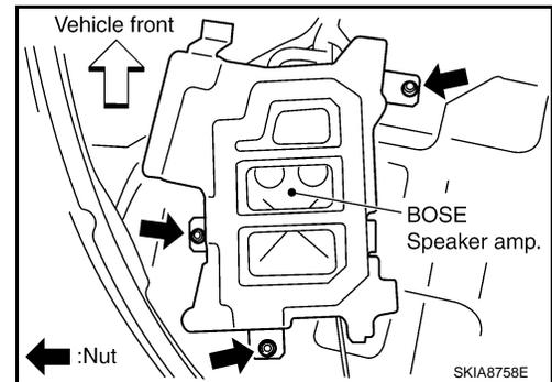
4. Remove bolts (4), and remove bracket.
