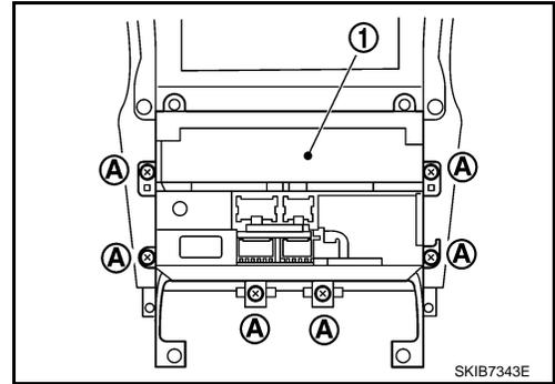
4. Remove screws (8), and remove bracket.
