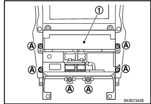
3. Remove screws (8), and remove bracket.
