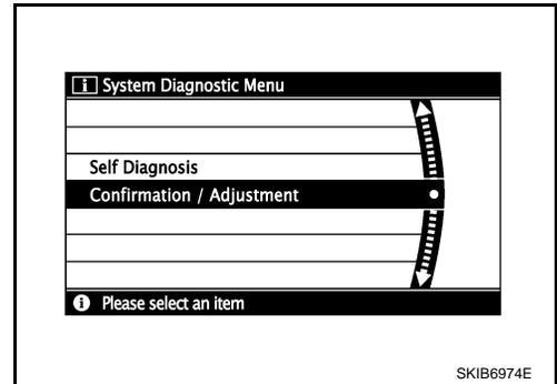
5. Each diagnosis is shown by selecting each screen switch on Confirmation/Adjustment screen.
