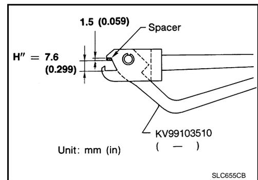
2. Check that when radiator plate pliers A [SST: KV99103510 ( — )] are closed dimension H'' is approx. 7.6 mm (0.299 in).
