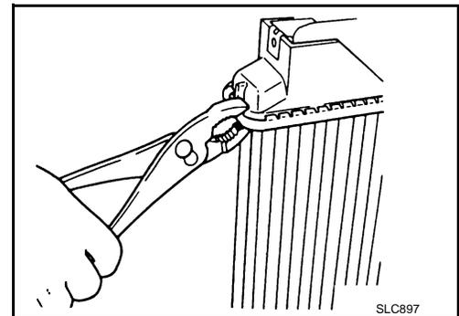
4. Check that the rim is completely crimped down.
