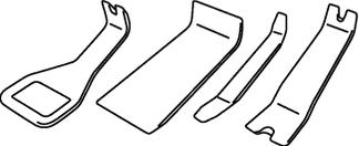
PIIB7923J  | Remove the clips, pawls and metal clips |
