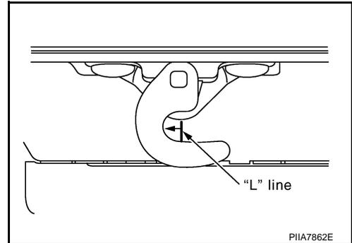
3. Adjust hook contact length by adjusting front lock rod length using front lock rod adjust bolt if "L" line is not exceeded in front lock hook, RH and LH.
