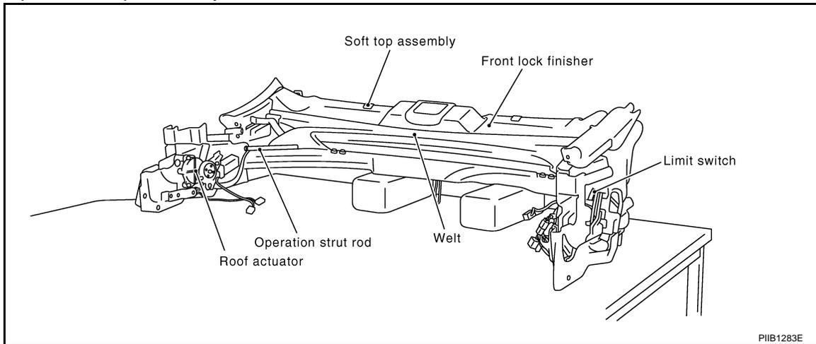
3. Remove roof actuator (RH/LH). Refer to [RF-101, "Removal and Installation of Roof Actuator"](#).
