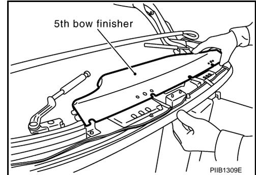
4. Remove rivets head of 5th bow finisher retainer.
