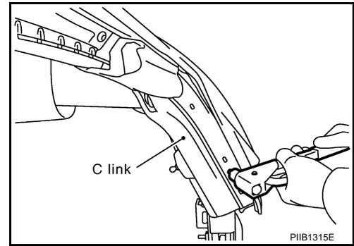
19. Align screw hole on soft top cover and the bottom of C link, and then tighten with screw.
