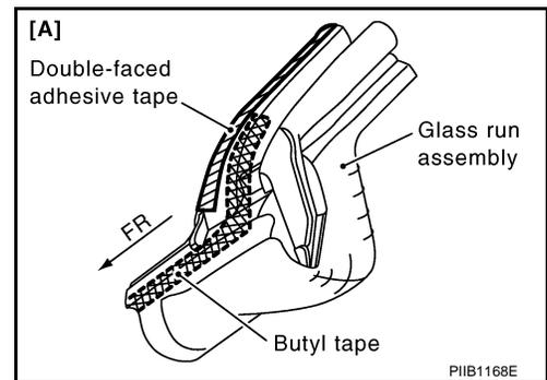
Water may be entering through connection between front pillar and front edge of soft top.
