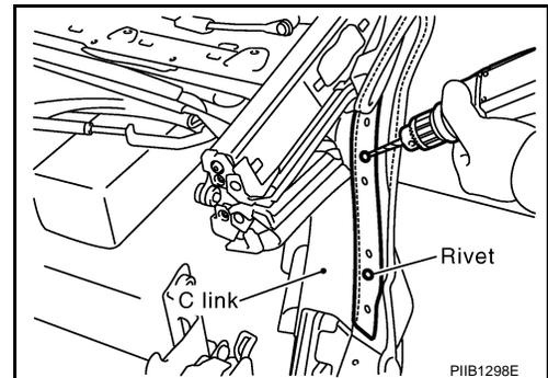
25. Cut EPT seal and remove screws on the bottom of C link.
