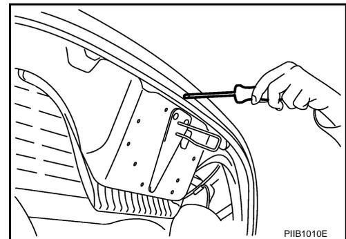
8. Drilling rivets attaching the soft top cover to 5th bow, then pull up the soft top cover bottom edge.
