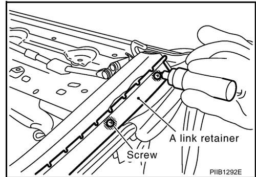
14. Remove screws, and then remove A link retainer.
