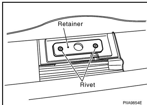
10. Drilling rivets under retainers by using 4 mm (0.16 in) diameter drill bit.
