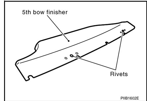
5. Replace retainers under 5th bow finisher with a new part.
