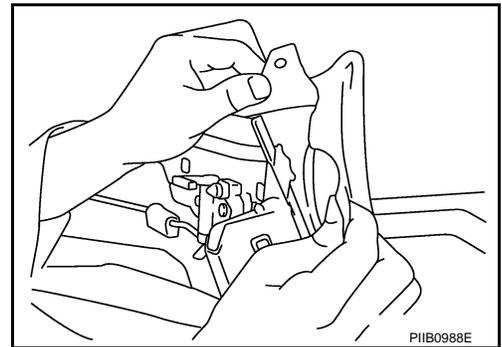
11. Align soft top cover hole and grommet hole at the 1st bow.
