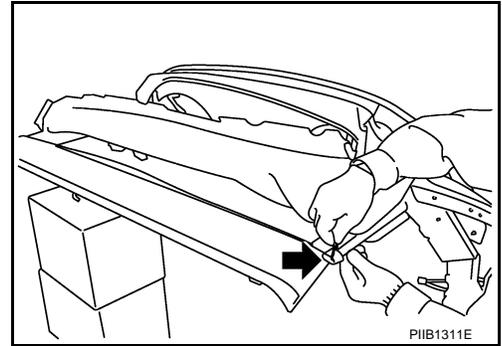
8. Tighten soft top cover wire rear bracket to C link with screw. (Face tension wire outside.)
