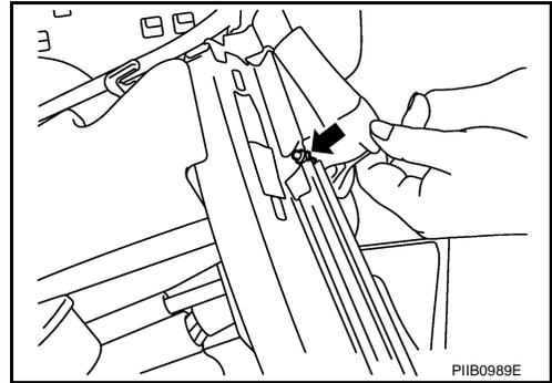
32. Remove soft top cover wire rear bracket from C link.
