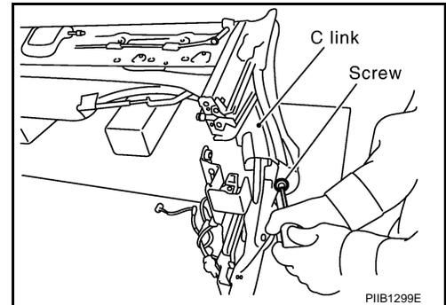
20. Close 5th bow then install 5th bow retainer with screws.
