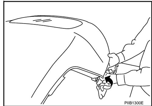
29. Open harness connector cover, and then disconnect defogger harness connector from terminal.
