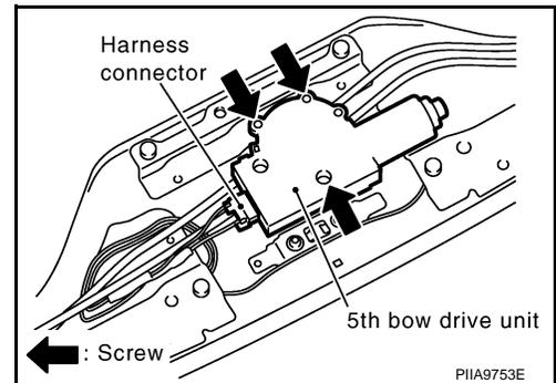
18. Remove 5th bow drive unit and rails together from 5th bow by removing screws.
