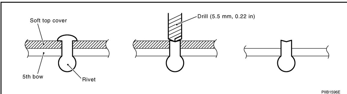
24. Close soft top, and then Shave rivets head and of C link by using a drill.
