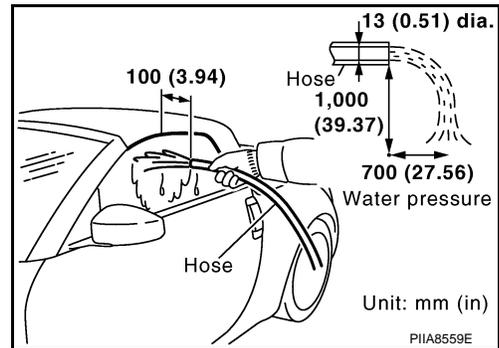
4. Visually check for water leakage.
