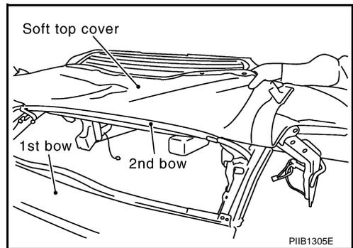
35. Pull up 2nd bow retainer by using a screwdriver, and then remove soft top cover from 2nd bow.
