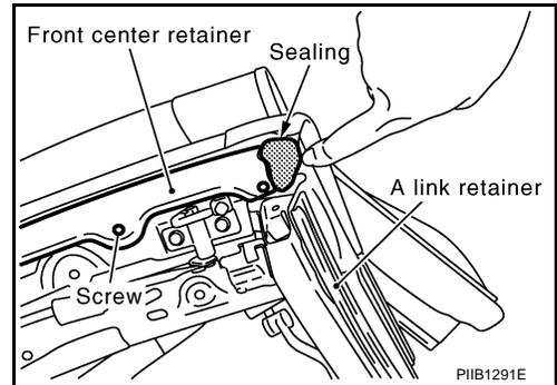
12. Remove screws, and then remove front center retainer.
