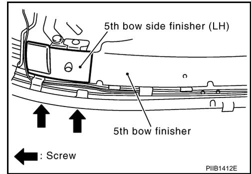
3. Remove clips, and then remove 5th bow finisher.
